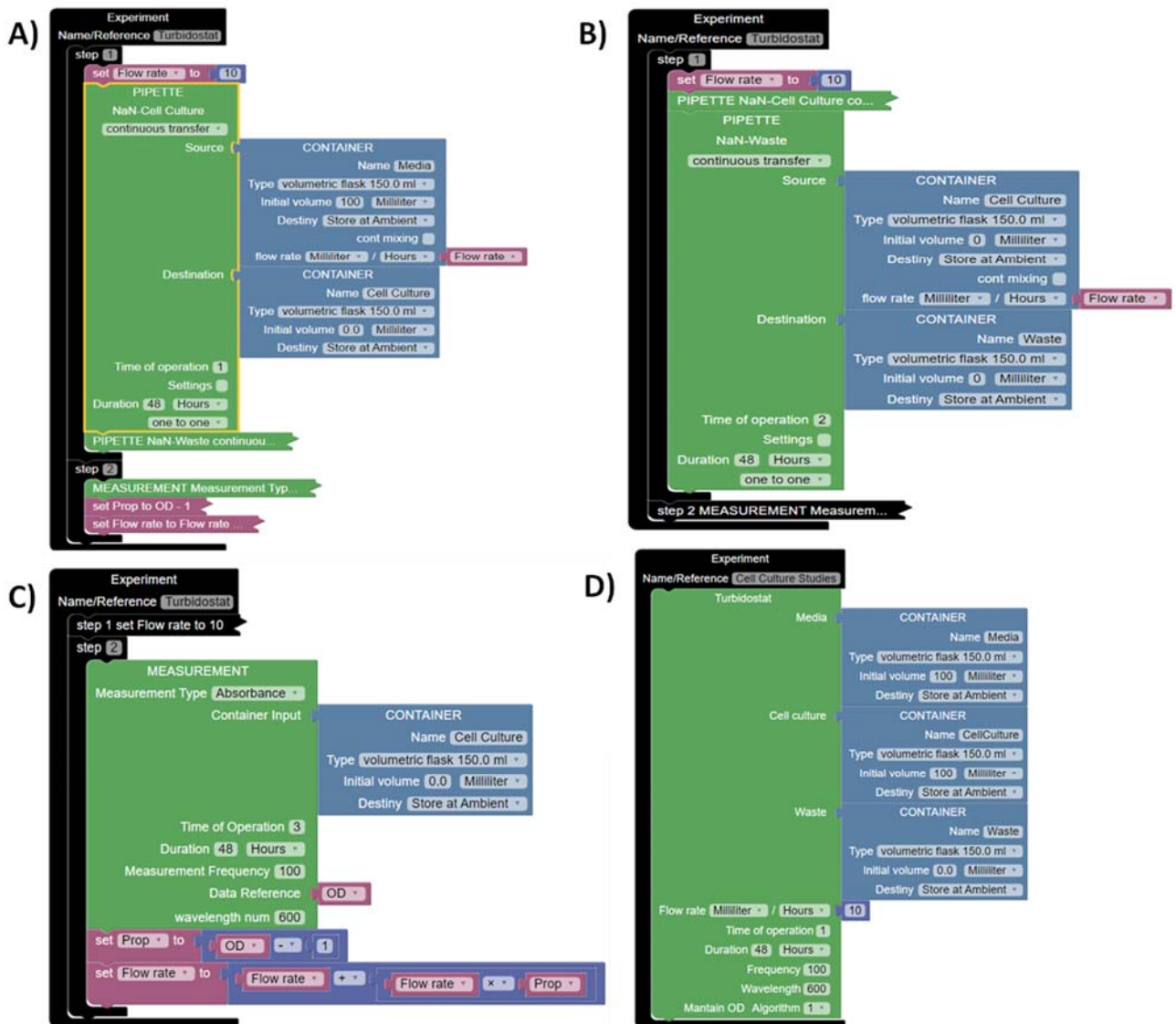
Supplementary Figure 2: Programming a Turbidostat using BioBlocks - A, B and C show how a Turbidostat can be programmed using general BioBlocks. They are shown in three parts so that user can observe all the steps in the protocol. The Blocks have been selectively minimized in all the three figures for the sake of viewing (A, B, C). D shows a simplified new BioBlock to program a Turbidostat. It has the same functionality of the protocol as shown in A,B and C. Simple BioBlocks with complex underlying functionality can be created to ease specification of complex protocols.
