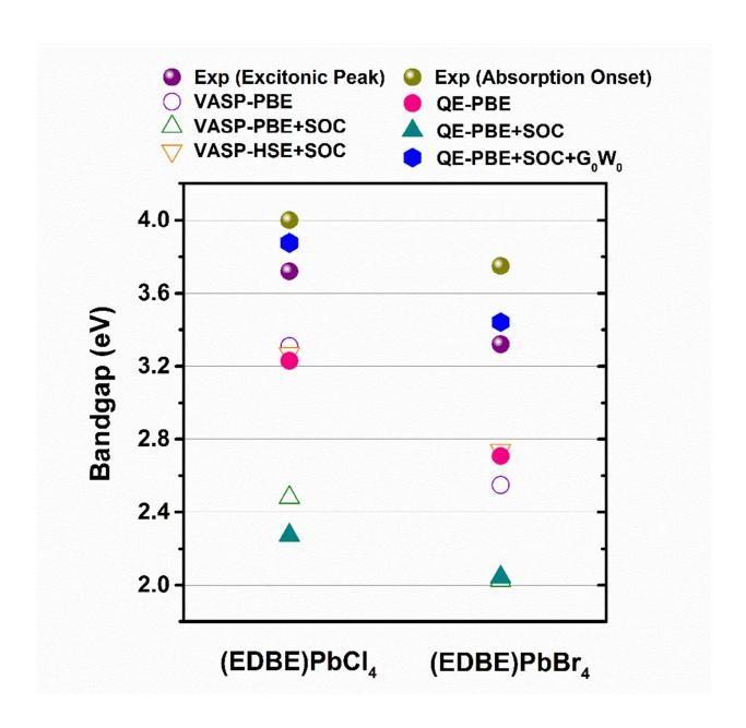
**Figure S3.** Bandgaps calculated using different methodologies (PBE, PBE+SOC, HSE+SOC, and PBE+SOC+G0W0) for the two-dimensional perovskites (EDBE)PbCl<sub>4</sub> and (EDBE)PbBr<sub>4</sub>.
