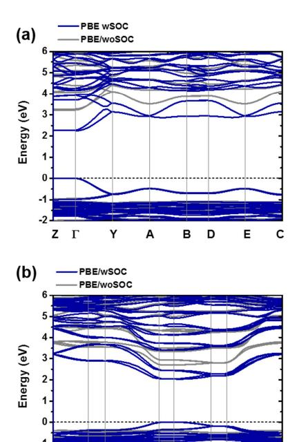
**Figure S2.** Band structures of the two-dimensional perovskites (a) (EDBE)PbCl<sub>4</sub> and (b) (EDBE)PbBr<sub>4</sub>, calculated with and without consideration of spin-orbit coupling at the PBE level, used for the evaluation of the optical response (Quantum Espresso code).
