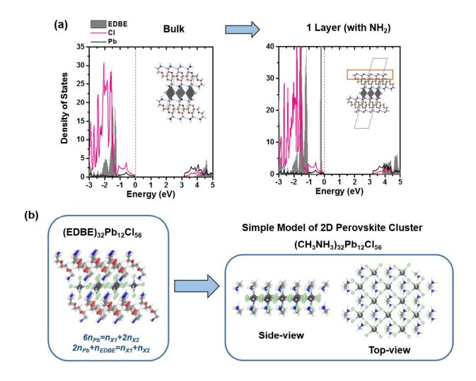
**Figure S4.** (a) Projected densities of states of (EDBE)PbCl<sub>4</sub> in the bulk and for a single layer with NH<sub>2</sub> terminations. (b) Molecular structures of the (EDBE)<sub>32</sub>Pb<sub>12</sub>Cl<sub>56</sub> cluster and corresponding simplified model of (CH<sub>3</sub>NH<sub>3</sub>)<sub>32</sub>Pb<sub>12</sub>Cl<sub>56</sub>.
