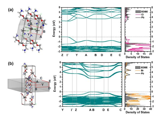
**Figure S1.** Band structures and densities of states of the two-dimensional perovskites: (a) (EDBE)PbCl<sub>4</sub> and (b) (EDBE)PbBr<sub>4</sub>, calculated at the HSE+SOC level (VASP code).
