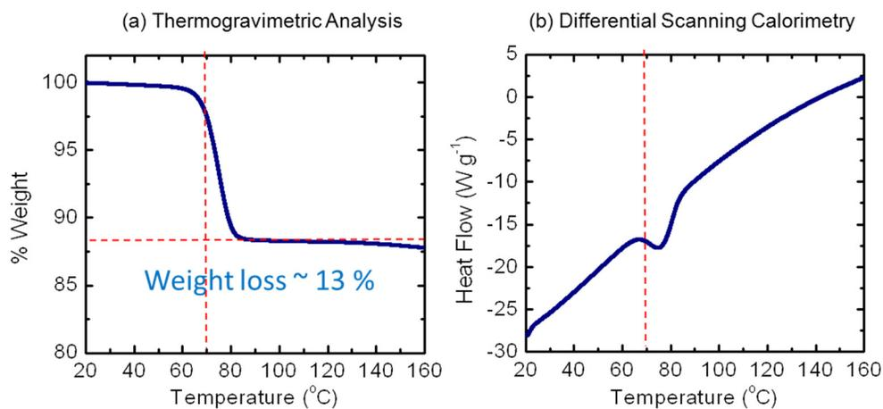
**Figure S1.** (a) TGA and (b) DSC Measurements on **2a**·MeCN. The loss of 1.0 mol MeCN from **2a**·MeCN requires a 12.4 % weight loss, in good agreement with the value of 13% obtained experimentally. The temperature of phase transition by DSC matches that obtained by TGA.
