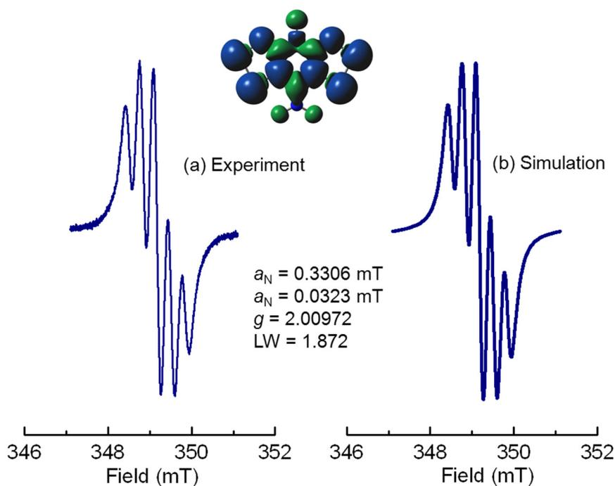
**Figure S2.** (a) Experimental and (b) simulated (with Winsim) EPR spectrum of **2a** in toluene (at  $\nu=9.821796$  GHz). The UB3LYP/6-311G(d,p) spin density distribution is also shown.
