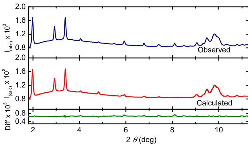
**Figure S5.** Powder diffraction pattern for **2a**·MeCN at 4.4 GPa.
