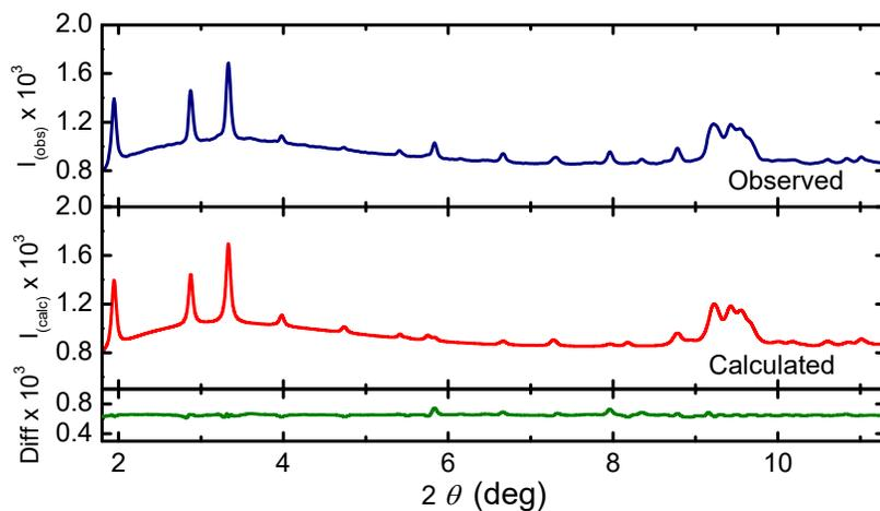
**Figure S4.** Powder diffraction pattern for **2a**·MeCN at 2.0 GPa.
