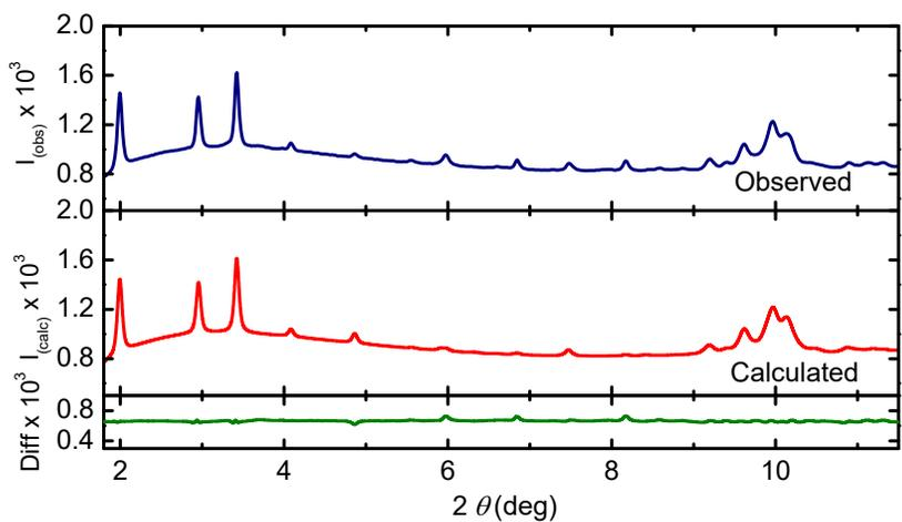
**Figure S6.** Powder diffraction pattern for **2a**·MeCN at 6.1 GPa.
