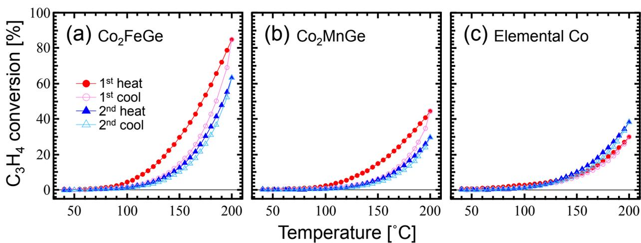
**Figure S3.** Conversion of  $C_3H_4$  in hydrogenation of propyne ( $C_3H_4$ ) by (a)  $Co_2FeGe$ , (b)  $Co_2MnGe$ , and (c) elemental Co. Data points were divided among thermal processes as shown by legend in (a). Heating: filled symbols, Cooling: open symbols, 1st cycle: red and pink circles, 2nd cycle: deep and pale blue triangles.
