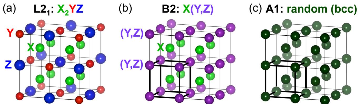
**Figure S1.** Crystal structures of (a) L2<sub>1</sub> phase and typical disordered phases in Heusler alloys: (b) B2 and (c) A1. B2 phase is disordered between Y and Z but ordered between X and (Y, Z). A1 phase is a completely disordered (random) structure (bcc structure). Unit cells of B2 and A1 are shown by thicker lines in (b) and (c). Figures were drawn using VESTA.<sup>2</sup>
