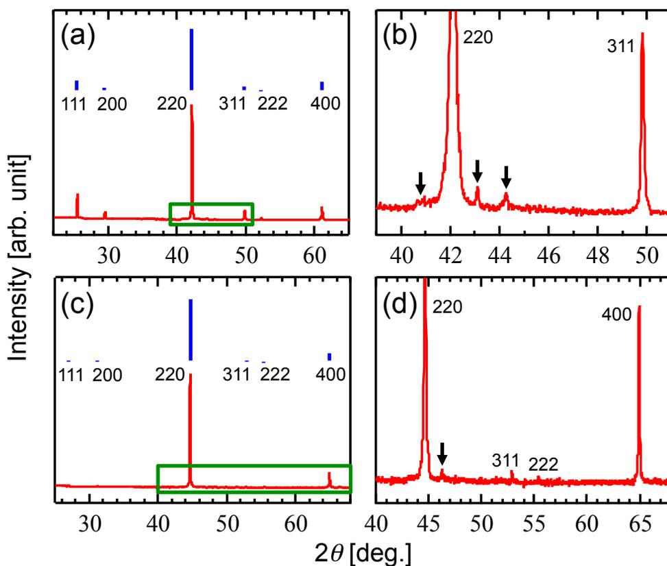
**Figure S2.** XRD patterns of (a, b) Co<sub>2</sub>TiSn and (c, d) Co<sub>2</sub>FeGe. (b) and (d) are magnified images in areas enclosed by green boxes in (a) and (c), respectively. Reflection indices are based on L2<sub>1</sub> structure. Blue bars in (a) and (c) are calculated peaks for each material. Arrows in (b) and (d) indicate peaks of extra phases.
