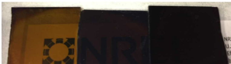
Fig. S1. CdTe films of three different thicknesses used as optical filters on conductive glass.
