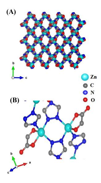
**Figure S2.** The pore structure (A) and local crystal structure (B) of  $ZOTW_x(1h)deCO_2$  simulated using the molecular structure of oxalate ion by the Rietveld method.
