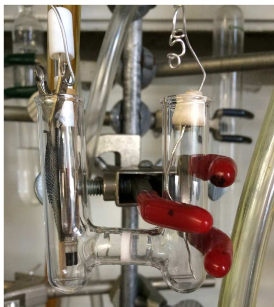
Figure S42. Picture of the small-volume H-cell for controlled potential electrolysis.
