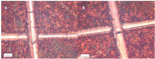
Figure S1. Pictures of iCVD coated plasma etched copper before (A) and after (B) removal of the scotch tape during the adhesion test. The test was conducted according to ASTM D 3359. There is no evidence of flakes or coating peeling off after the test, thus the adhesion between coating and substrate was classified as 5B, very good adhesion. Both scale bars correspond to 50  $\mu$ m.
