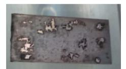
Figure S3. Image of a copper sample after exposure to  $O_2$  plasma at 150 W for 5 minutes. A dark layer of copper oxide was formed after the  $O_2$  plasma. The bright spots observed correspond to the copper substrate where the oxide layer was peeled off. The oxide layer was easily removed because of the poor adhesion with the substrate.
