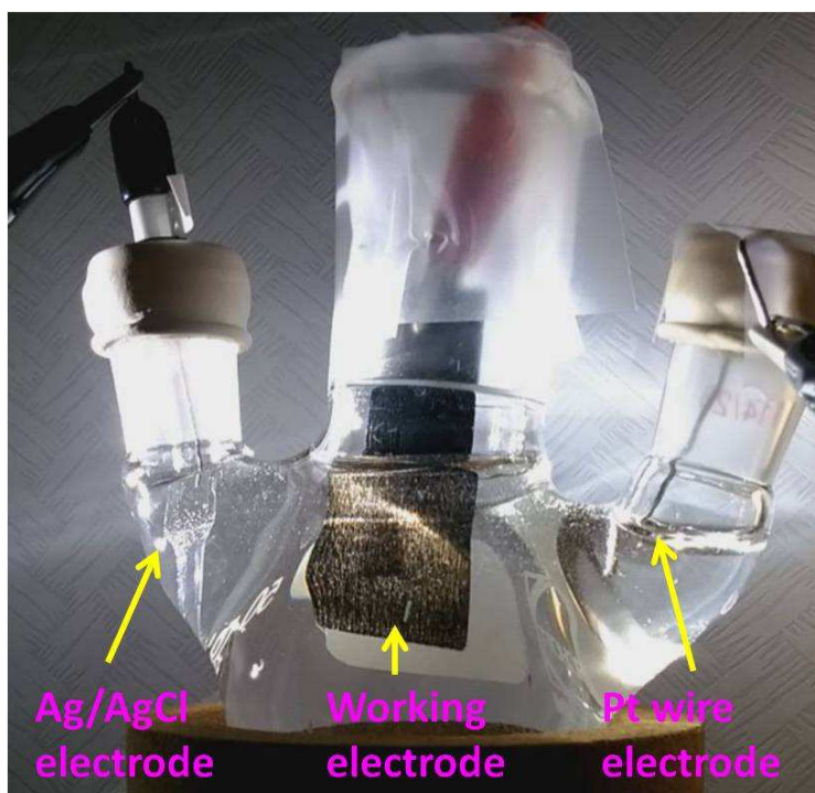
Figure S9. Digital image of the electrocatalytic measurement in a three-electrode glass cell with P,S-CNS grown on carbon fiber paper directly used as the working electrode.
