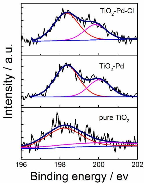
**Figure S8.** XPS Cl 2p spectra of as-prepared pure  $\text{TiO}_2$ ,  $\text{TiO}_2\text{-Pd}$  and  $\text{TiO}_2\text{-Pd-Cl}$ .
