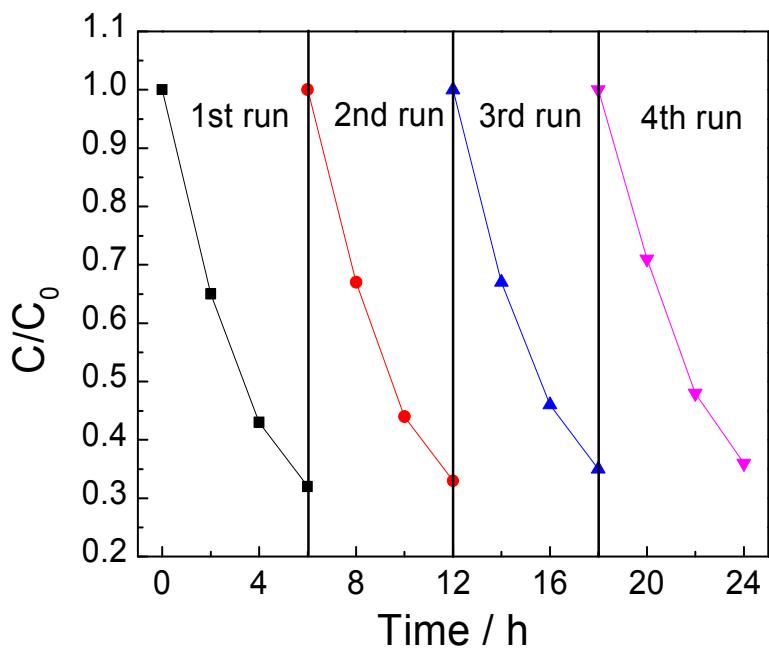
**Figure S11.** Reusability of  $\text{TiO}_2\text{-Pd-Cl}$  for the visible photocatalytic degradation of 4-BrPh ( $5 \times 10^{-5} \text{ mol L}^{-1}$ ).
