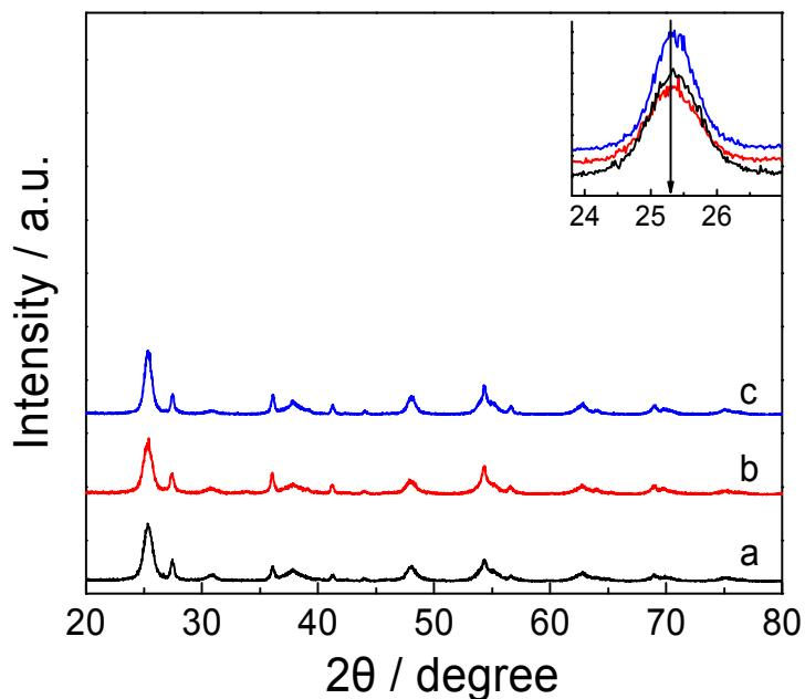
**Figure S6.** XRD patterns of the as-prepared samples. (a) pure TiO<sub>2</sub>, (b) Pd-TiO<sub>2</sub>, (c) TiO<sub>2</sub>-Pd-Cl.
