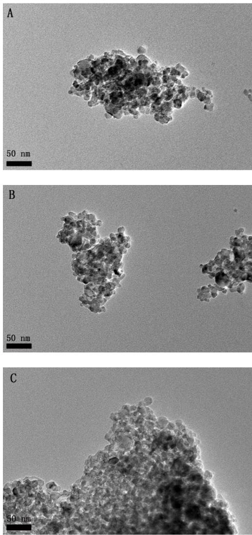
**Figure S7.** TEM images of the as-prepared samples: pure TiO<sub>2</sub> (A), TiO<sub>2</sub>-Pd (B) and TiO<sub>2</sub>-Pd-Cl (C).
