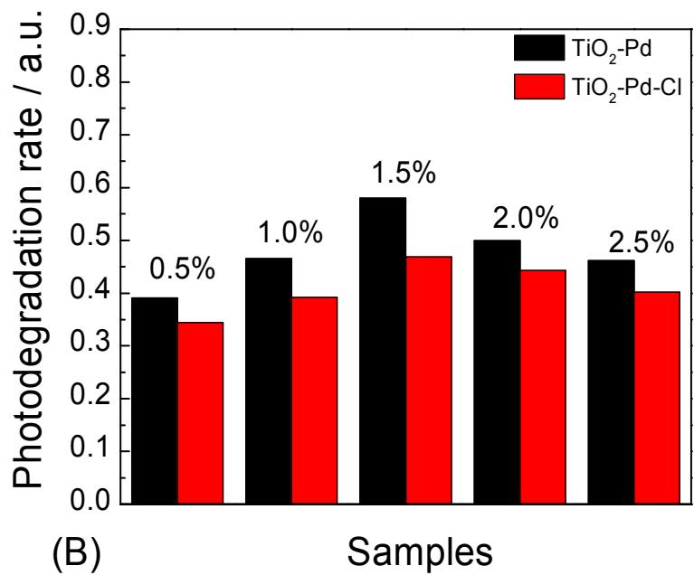
**Figure S5.** Photodegradation rate of 4-BrPh (A) and phenol (B) in aqueous suspension using catalysts with different molar ratio of  $\text{Pd}^{2+}$  to  $\text{Ti}^{4+}$  under visible light irradiation ( $\lambda > 420 \text{ nm}$ ) for 8 h.
