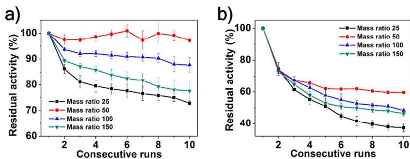
**Figure S6.** Effect of ConA on the reusability of immobilized enzyme on AC, and mass ratio means mass ratio of ConA to AC ( $\text{mg g}^{-1}$ ).
