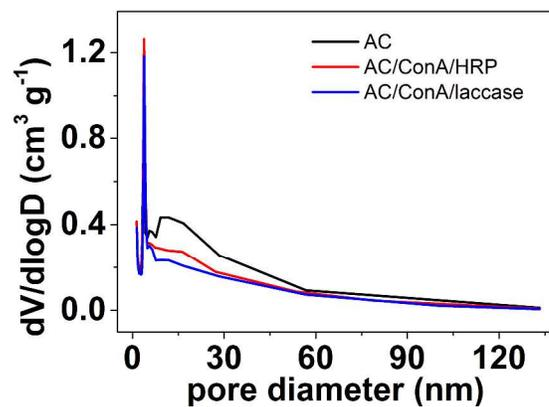
**Figure S4.** Pore size distribution of 20-40 mesh AC before and after protein adsorption.
