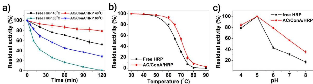
**Figure S9.** Stability characterization of AC/ConA/HRP and free HRP. (a) thermostability in 60 °C and 65 °C; (b) effect of temperature on the apparent activity; (c) effect of pH on the apparent activity.
