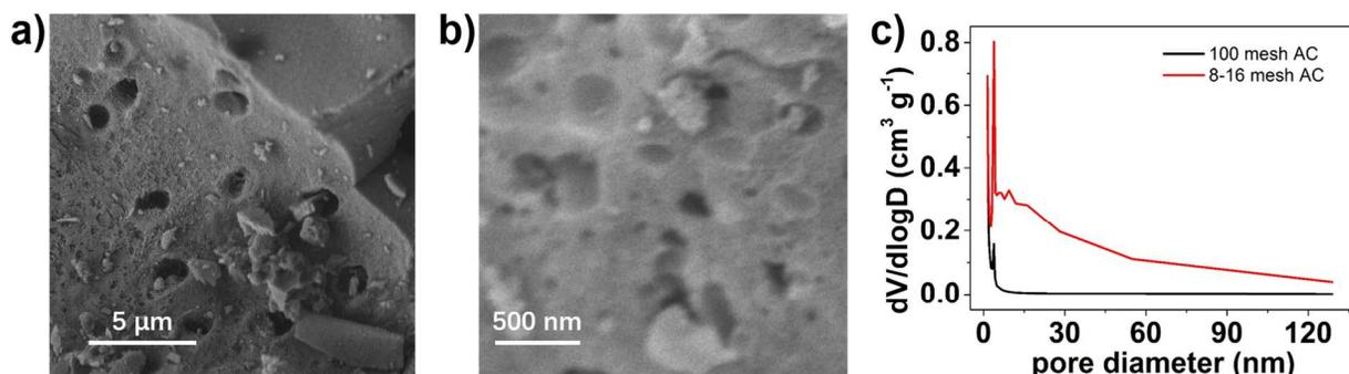
**Figure S8.** SEM images of (a) 8-16 mesh AC and (b) 100 mesh AC; (c) pore size distribution of 8-16 mesh AC and 100 mesh AC.
