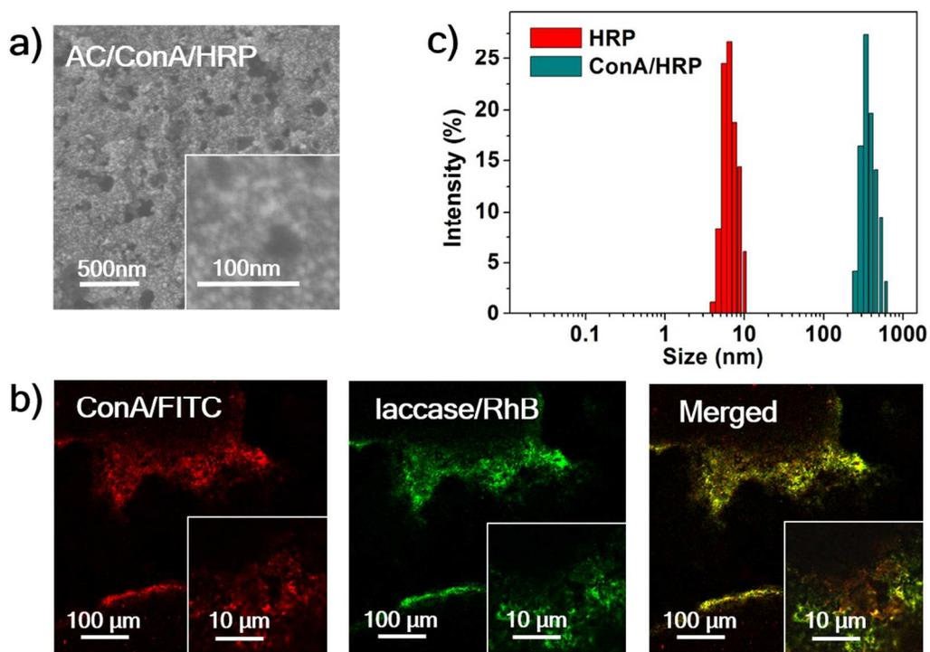
**Figure S3.** Structure characterizations of HRP immobilized on AC coated with ConA. (a) SEM (inset: high-resolution SEM); (b) laser confocal microscopy, in which HRP were labelled with RhB (red) and ConA was labelled with FITC (green), respectively; (c) DLS of HRP and ConA/HRP.
