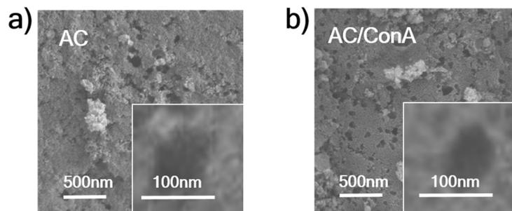
**Figure S2.** SEM images of (a) AC and (b) AC/ConA (inset: high-resolution SEM)
