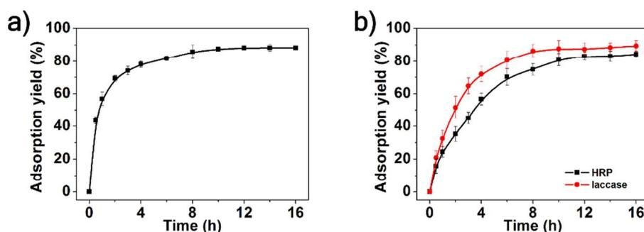
**Figure S1.** Adsorption kinetic curves of (a) ConA and (b) laccase and HRP to AC
