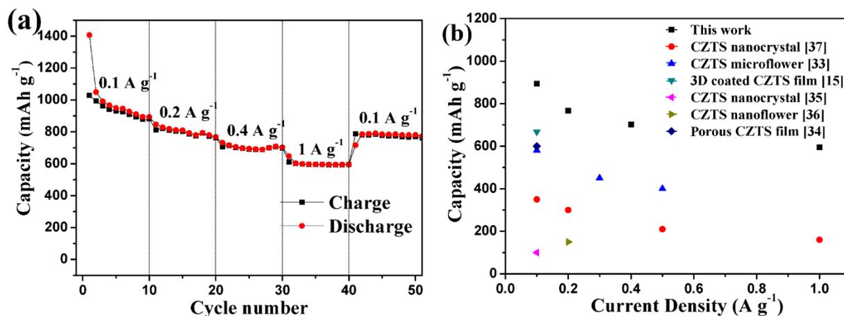
**Figure S4.** (a) Rate capability of CZTS thin film (300 nm) and (b) comparison with other reports.
