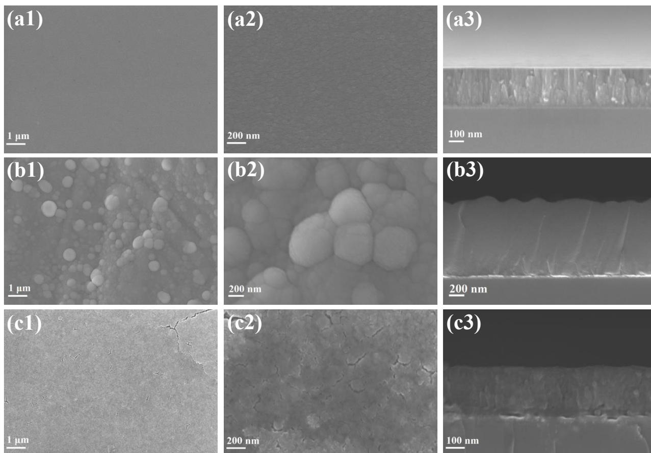
**Figure S1.** Surface and cross section SEM images of (a1-a3) thin SnO<sub>2</sub>, (b1-b3) thick CZTS and (c1-c3) LiCoO<sub>2</sub> films.
