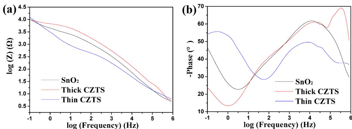
**Figure S5.** Bode plots of (a) Z-Frequency and (b) Phase-Frequency curves.
