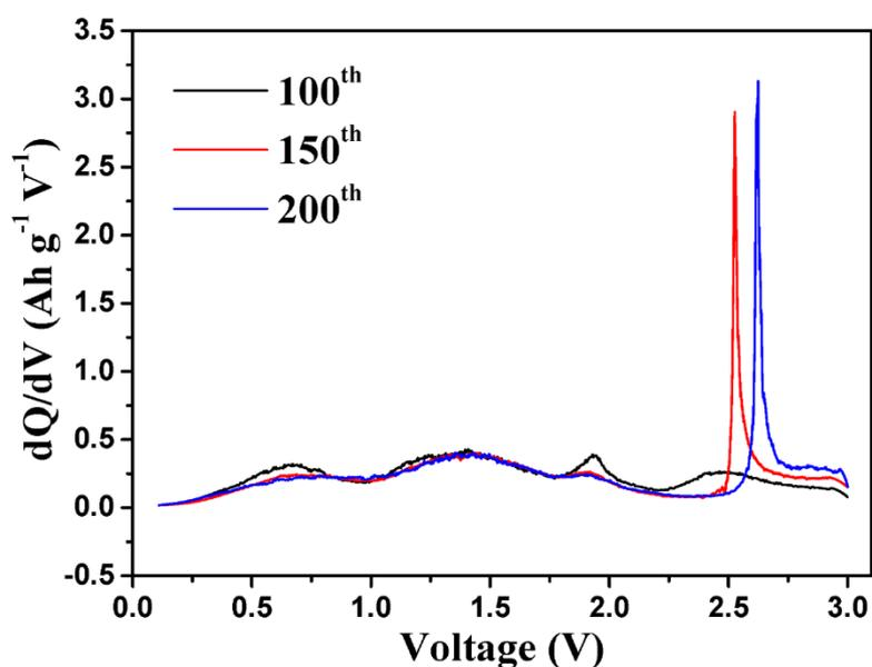
**Figure S3.** Differential charge plots of CZTS thin film (300 nm) in 100<sup>th</sup>, 150<sup>th</sup> and 200<sup>th</sup> cycles.
