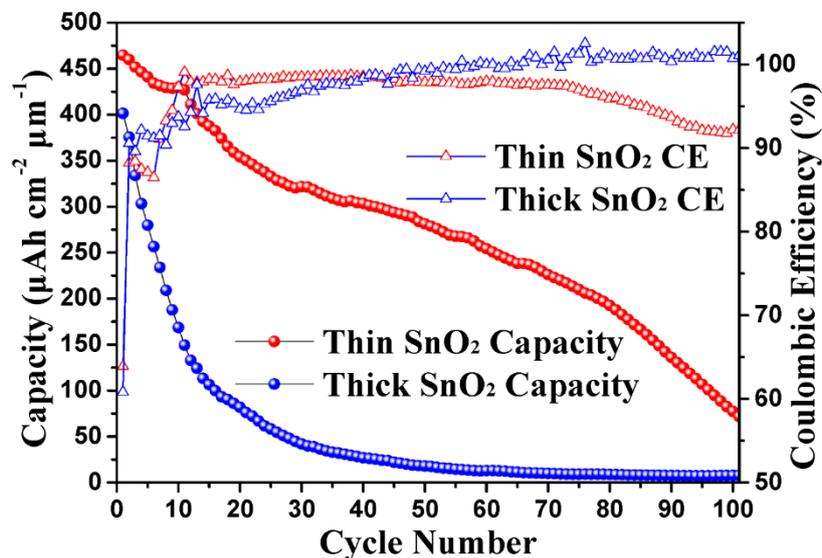
**Figure S2.** Cycle performance of thin and thick  $\text{SnO}_2$  films in half-cells based on charge capacity.
