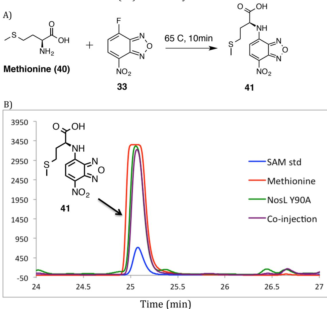
**Figure S12:** Analysis of the reaction mixture for SAM derived amine products. A) Scheme depicting the derivatization reaction between methionine and NBD-F. B) HPLC analysis at 475 nm of the enzymatic reaction after treatment with NBD-F. The observed reaction product comigrated with an authentic sample of **41**.
