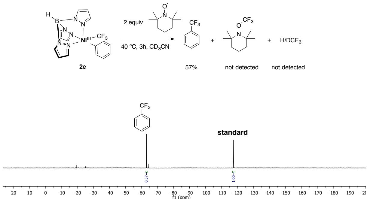
**Figure S14.** <sup>19</sup>F NMR spectrum of **2e** and TEMPO after heating at 40 °C for 3 h. Standard = 4,4'-difluorobiphenyl.
