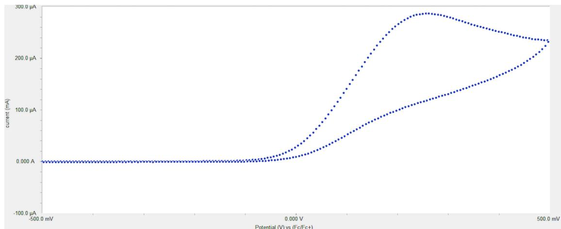
**Figure S39.** Cyclic voltammogram of **1f** [0.01 M] with 0.1 M NBu<sub>4</sub>PF<sub>6</sub> in MeCN at a scan rate of 100 mV/s.
