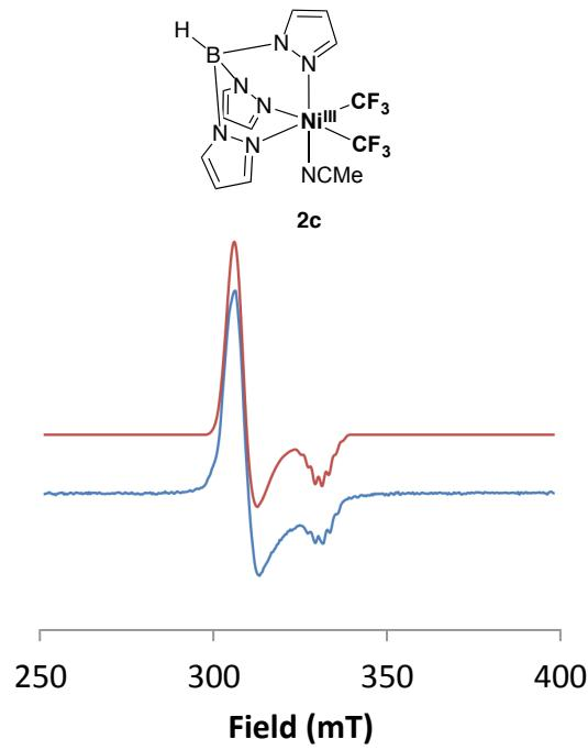
**Figure S4.** EPR spectrum of **2c** (bottom/blue) and the simulated spectrum (top/red). Fit using the following parameters:  $g_x = 2.18$ ,  $g_y = 2.15$ ,  $g_z = 2.00$ ,  $A_N(\text{N}) = 21\text{G}$ ,  $A_N(\text{N}') = 18\text{G}$ .
