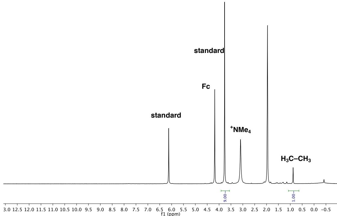
**Figure S6.** <sup>1</sup>H NMR spectrum of the crude reaction mixture after oxidation of **1d** with FcBF<sub>4</sub>. Standard = 1,3,5-trimethoxybenzene
