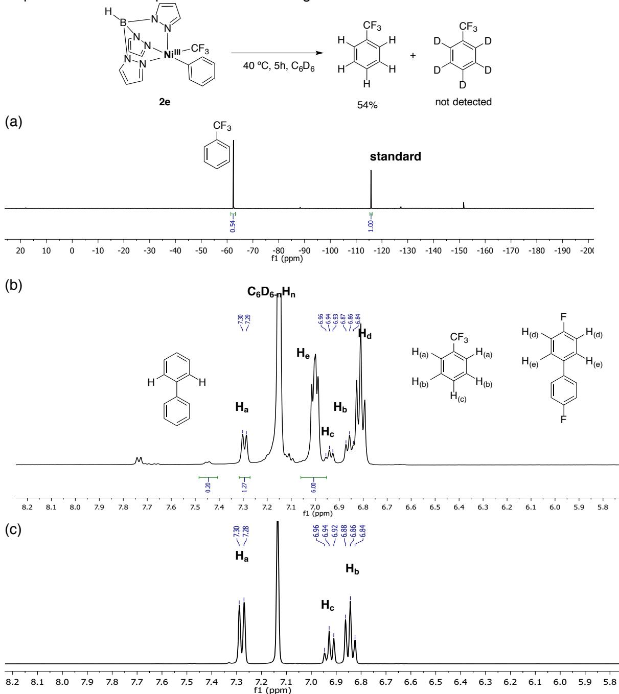
**Figure S15.** (a)  $^{19}\text{F}$  NMR spectrum and (b)  $^1\text{H}$  NMR spectrum of the crude reaction mixture after heating **2e** at 40 °C for 5 h; (c)  $^1\text{H}$  NMR spectrum of authentic  $\text{C}_6\text{H}_5\text{CF}_3$  in  $\text{C}_6\text{D}_6$  for comparison.
