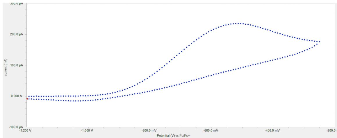
**Figure S34.** Cyclic voltammogram of **1d** [0.01 M] with 0.1 M NBu<sub>4</sub>PF<sub>6</sub> in MeCN at a scan rate of 500 mV/s.
