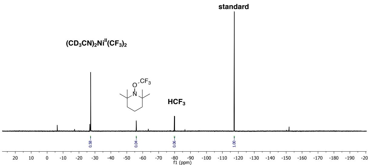
**Figure S13.** <sup>19</sup>F NMR spectrum of **2c** and TEMPO after heating at 70 °C for 8 h. Standard = 4,4'-difluorobiphenyl.
