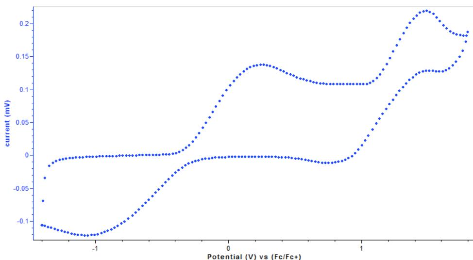
**Figure S31.** Cyclic voltammogram of **1c** [0.01 M] with 0.1 M NBu<sub>4</sub>PF<sub>6</sub> in MeCN at a scan rate of 250 mV/s.
