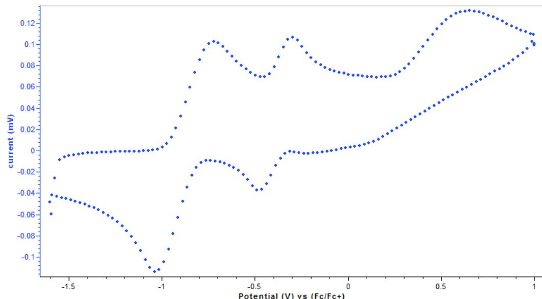
**Figure S28.** Cyclic voltammogram of **1b** [0.01 M] with 0.1 M NBu<sub>4</sub>PF<sub>6</sub> in MeCN at a scan rate of 250 mV/s with (C<sub>5</sub>Me<sub>5</sub>)<sub>2</sub>Fe added as internal standard.
