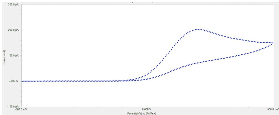
**Figure S38.** Cyclic voltammogram of **1f** [0.01 M] with 0.1 M  $\text{NBu}_4\text{PF}_6$  in MeCN at a scan rate of 50 mV/s.
