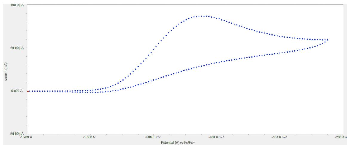
**Figure S32.** Cyclic voltammogram of **1d** [0.01 M] with 0.1 M  $\text{NBu}_4\text{PF}_6$  in MeCN at a scan rate of 50 mV/s.
