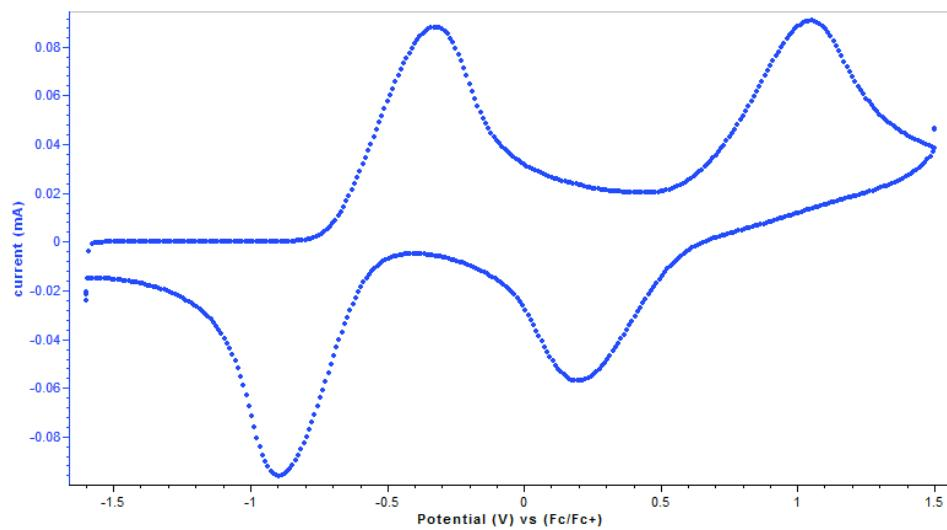
**Figure S36.** Cyclic voltammogram of **1e** [0.01 M] with 0.1 M NBu<sub>4</sub>PF<sub>6</sub> in MeCN at a scan rate of 100 mV/s.
