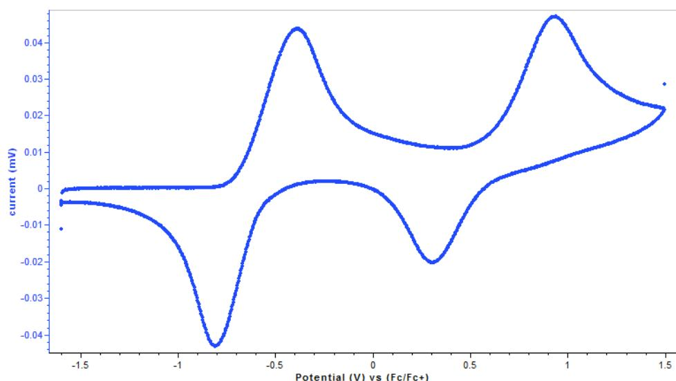
**Figure S35.** Cyclic voltammogram of **1e** [0.01 M] with 0.1 M  $\text{NBu}_4\text{PF}_6$  in MeCN at a scan rate of 50 mV/s.
