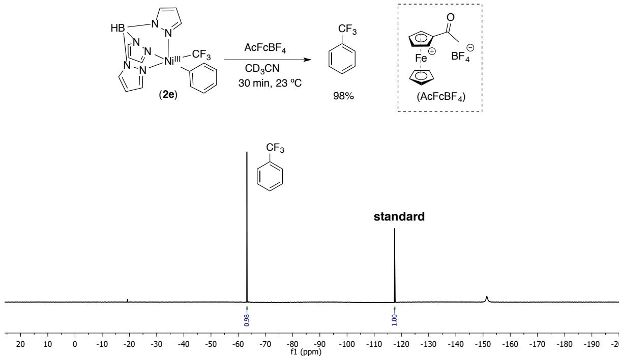
**Figure S17.** <sup>19</sup>F NMR spectrum of the crude reaction mixture 30 minutes after treating **2e** with 1 equiv of acetyl ferrocenium tetrafluoroborate.
