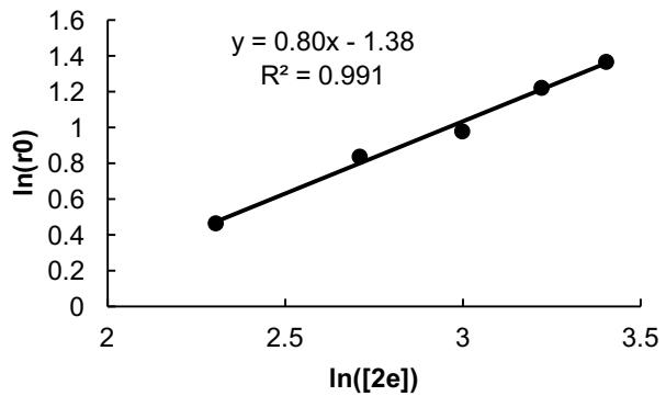
**Figure S21.** (a) Plot of initial rates of Ph-CF<sub>3</sub> formation versus [Ni] for Ph-CF<sub>3</sub> coupling from **2e** fit to  $y=a[X]^n$ . (b) A log-log plot of initial rate of Ph-CF<sub>3</sub> formation as a function of nickel concentration
