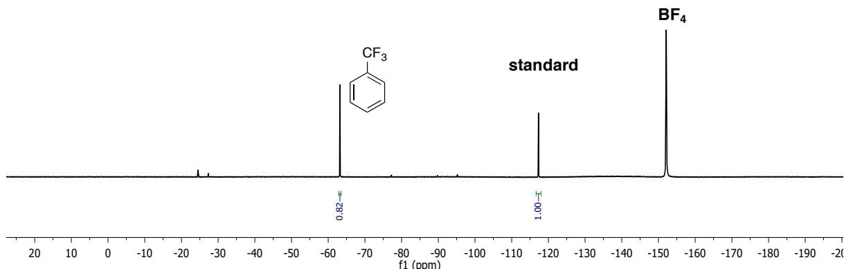
**Figure S18.** <sup>19</sup>F NMR spectrum of the crude reaction mixture after heating **2e** at 40 °C for 5 h in the presence of (a) 1 equiv of Cp<sub>2</sub>\*FeBF<sub>4</sub> or (b) 5 equiv of Cp<sub>2</sub>\*FeBF<sub>4</sub>.
