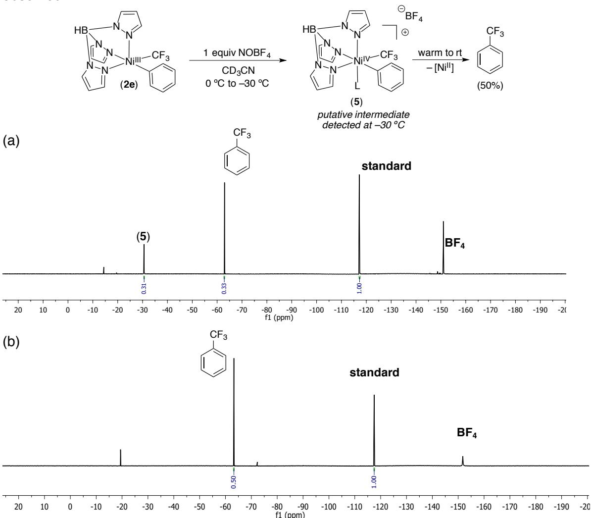
**Figure S16.**  $^{19}\text{F}$  NMR spectrum of **2e** when reacted with 1 equiv of  $\text{NOBF}_4$  at (a)  $-30$  °C after 1 min and (b) after warming to room temperature for 2 min
