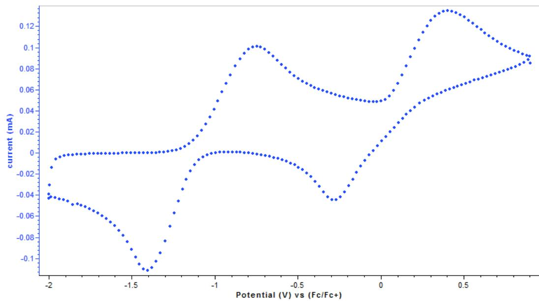
**Figure S25.** Cyclic voltammogram of **1a** [0.01 M] with 0.1 M NBu<sub>4</sub>PF<sub>6</sub> in MeCN at a scan rate of 250 mV/s.
