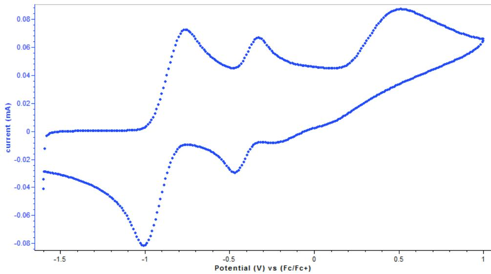
**Figure S27.** Cyclic voltammogram of **1b** [0.01 M] with 0.1 M NBu<sub>4</sub>PF<sub>6</sub> in MeCN at a scan rate of 100 mV/s with (C<sub>5</sub>Me<sub>5</sub>)<sub>2</sub>Fe added as internal standard.
