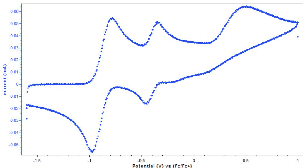
**Figure S26.** Cyclic voltammogram of **1b** [0.01 M] with 0.1 M  $\text{NBu}_4\text{PF}_6$  in MeCN at a scan rate of 50 mV/s with  $(\text{C}_5\text{Me}_5)_2\text{Fe}$  added as internal standard.
