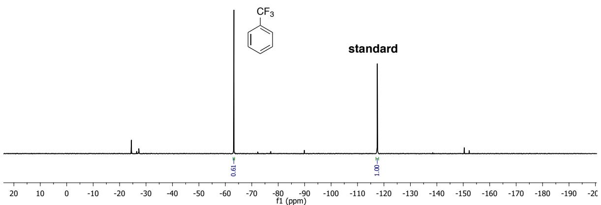
**Figure S12.** (a) A representative  $^{19}\text{F}$  NMR spectrum of the crude reaction mixture after heating **2e** at 80 °C for 5 min. Standard = 4,4-difluorobiphenyl.
