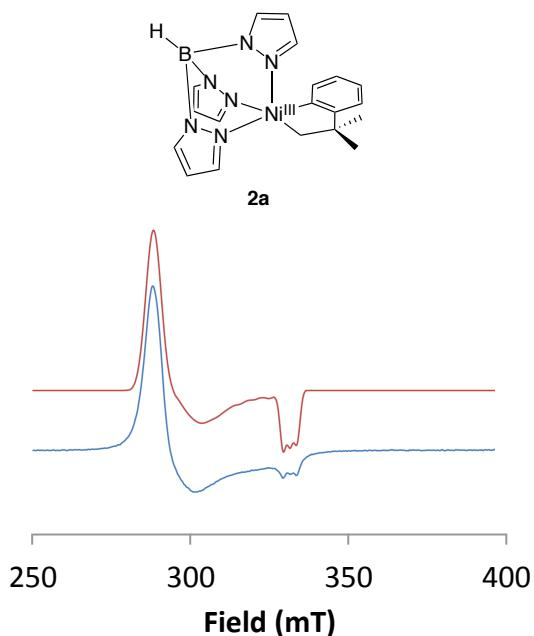
**Figure S2.** EPR spectrum of **2a** (bottom/blue) and the simulated spectrum (top/red). Fit using the following parameters:  $g_x = 2.29$ ,  $g_y = 2.25$ ,  $g_z = 2.01$ ,  $A_N = 21 \text{ G}$ .
