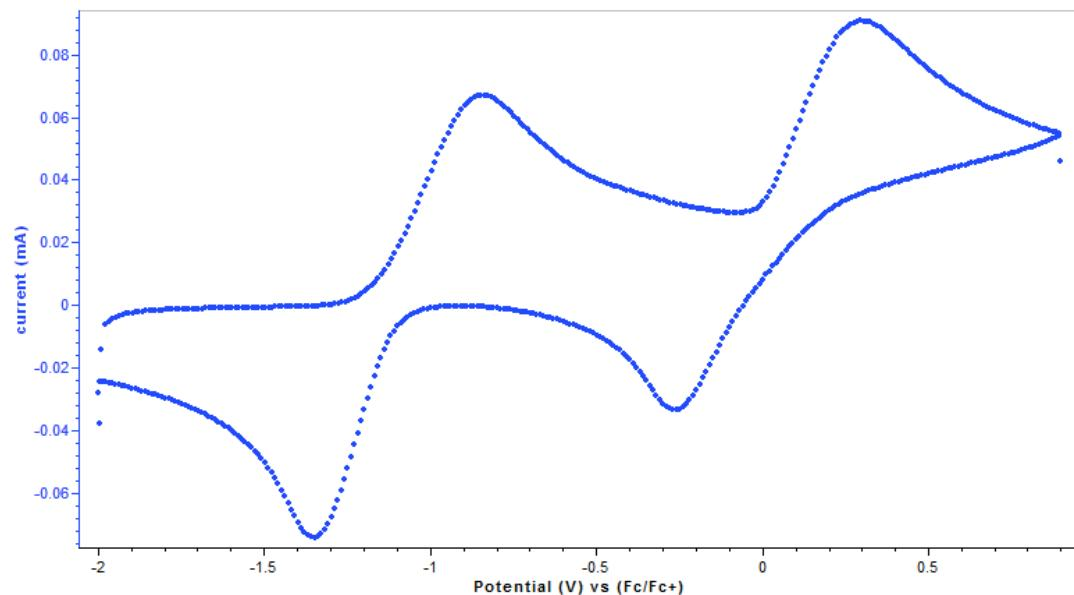
**Figure S24.** Cyclic voltammogram of **1a** [0.01 M] with 0.1 M NBu<sub>4</sub>PF<sub>6</sub> in MeCN at a scan rate of 100 mV/s.
