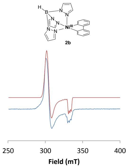
**Figure S3.** EPR spectrum of **2b** (bottom/blue) and the simulated spectrum (top/red). Fit using the following parameters:  $g_x = 2.20$ ,  $g_y = 2.19$ ,  $g_z = 2.01$ ,  $A_N = 19\text{G}$ .
