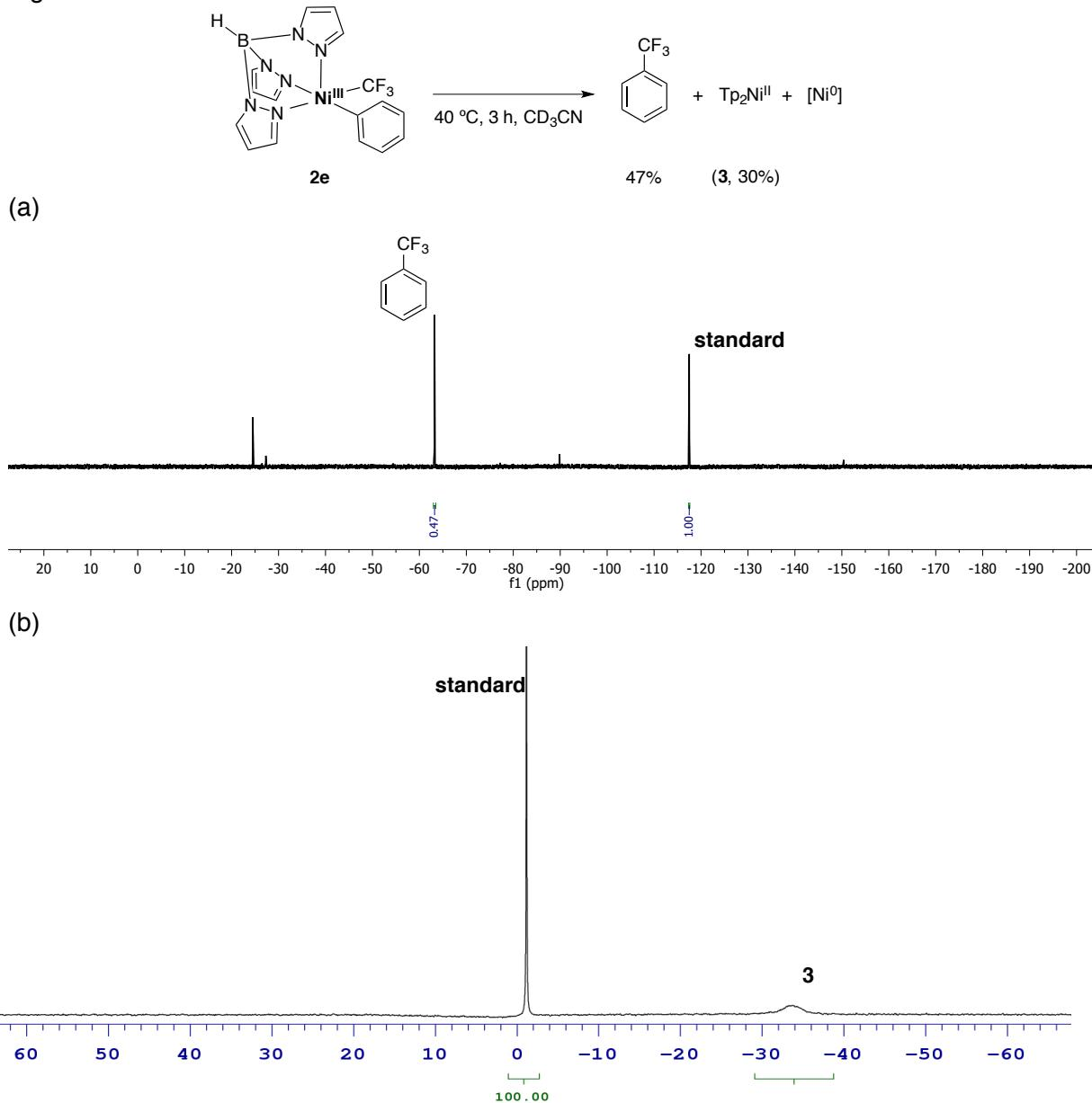
**Figure S11.** (a) <sup>19</sup>F NMR spectrum of the crude reaction mixture after heating **2e** at 40 °C for 3 h. Standard = 4,4'-difluorobiphenyl; (b) <sup>11</sup>B NMR spectrum of the reaction mixture after heating for 40 °C for 3 h. Standard = NBu<sub>4</sub>BF<sub>4</sub>
