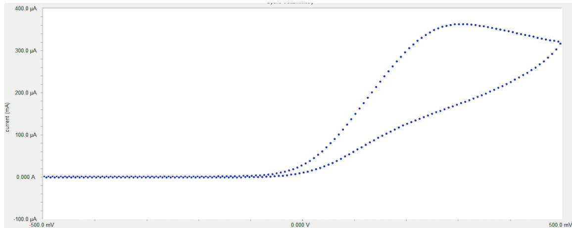
**Figure S40.** Cyclic voltammogram of **1f** [0.01 M] with 0.1 M NBu<sub>4</sub>PF<sub>6</sub> in MeCN at a scan rate of 500 mV/s.
