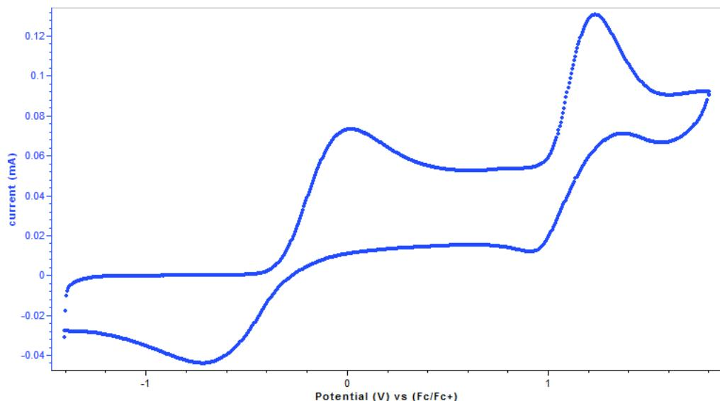
**Figure S29.** Cyclic voltammogram of **1c** [0.01 M] with 0.1 M  $\text{NBu}_4\text{PF}_6$  in MeCN at a scan rate of 50 mV/s .
