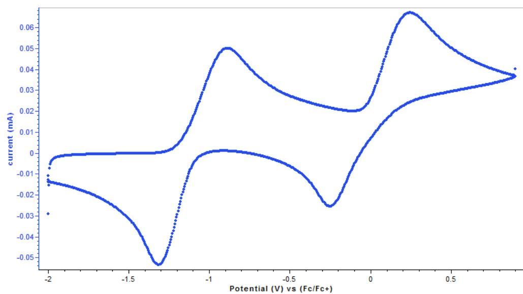
**Figure S23.** Cyclic voltammogram of **1a** [0.01 M] with 0.1 M NBu<sub>4</sub>PF<sub>6</sub> in MeCN at a scan rate of 50 mV/s
