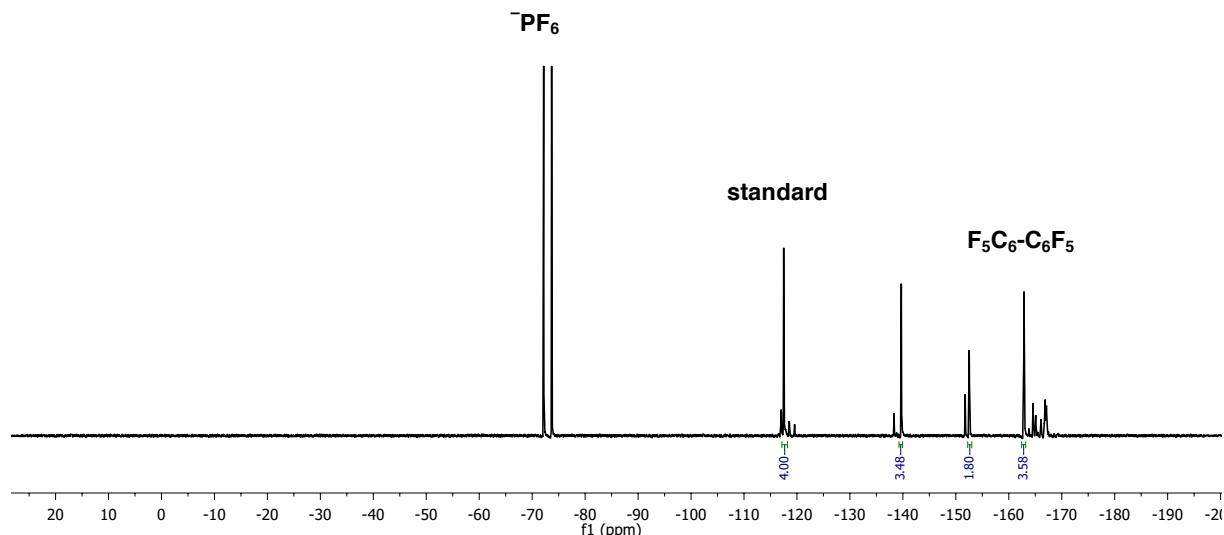
**Figure S7.** <sup>19</sup>F NMR spectrum of the crude reaction mixture after oxidation of **1f** with FcPF<sub>6</sub>. Standard = 4,4'-difluorobiphenyl.
