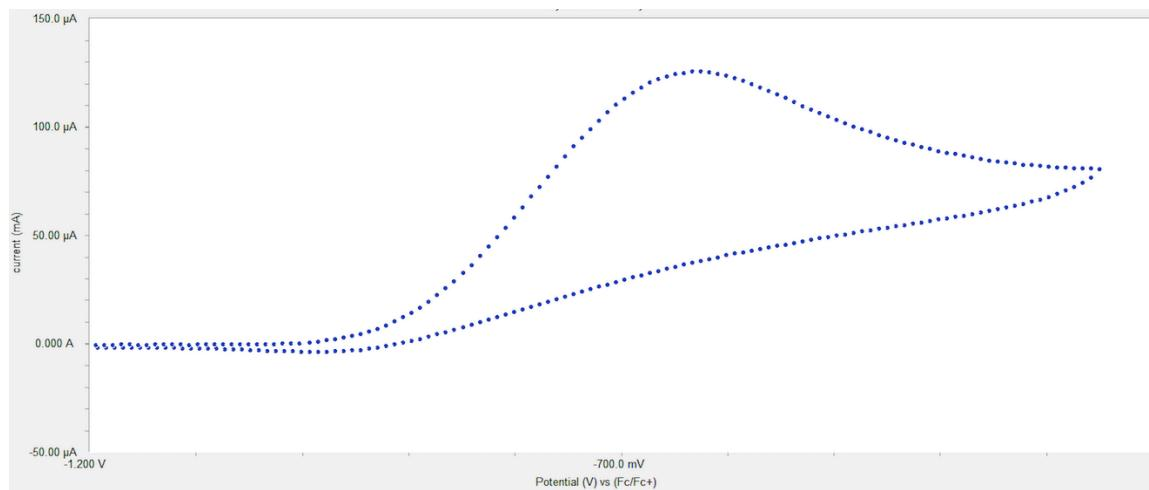
**Figure S33.** Cyclic voltammogram of **1d** [0.01 M] with 0.1 M NBu<sub>4</sub>PF<sub>6</sub> in MeCN at a scan rate of 100 mV/s.
