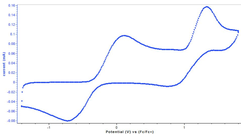
**Figure S30.** Cyclic voltammogram of **1c** [0.01 M] with 0.1 M NBu<sub>4</sub>PF<sub>6</sub> in MeCN at a scan rate of 100 mV/s with (C<sub>5</sub>Me<sub>5</sub>)<sub>2</sub>Fe added as internal standard..
