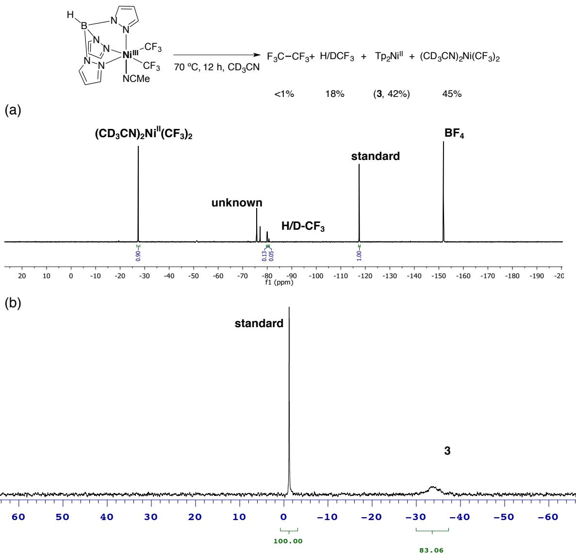
**Figure S10.** (a) <sup>19</sup>F NMR spectrum of the crude reaction mixture after heating **2c** at 70 °C for 12 h. Standard =4,4'-difluorobiphenyl; (b) <sup>11</sup>B NMR of the reaction mixture after heating for 70 °C for 12 h. Standard = NBu<sub>4</sub>BF<sub>4</sub>.
