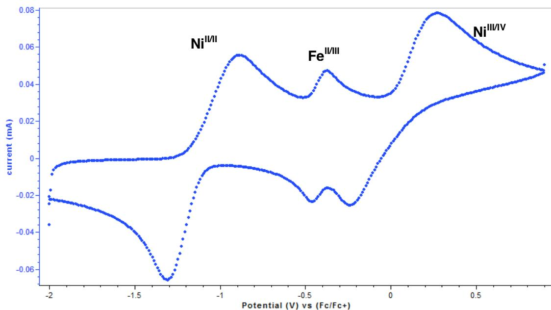
**Figure S22.** Cyclic voltammogram of **1a** [0.01 M] with 0.1 M  $NBu_4PF_6$  in MeCN at a scan rate of 50 mV/s with  $(C_5Me_5)_2Fe$  added as the internal standard.
