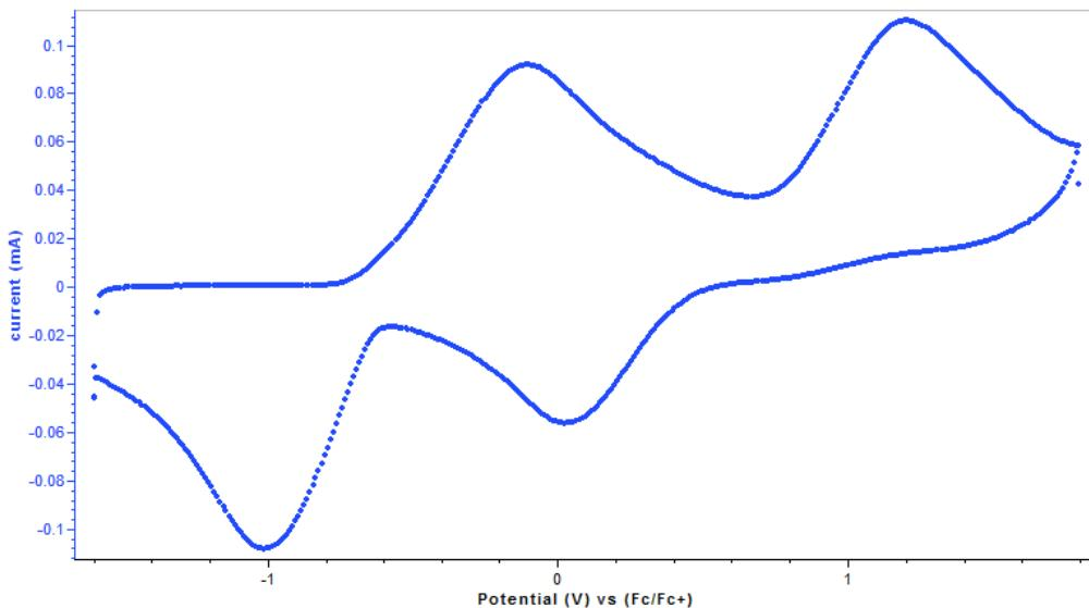
**Figure S37.** Cyclic voltammogram of **1e** [0.01 M] with 0.1 M NBu<sub>4</sub>PF<sub>6</sub> in MeCN at a scan rate of 250 mV/s.
