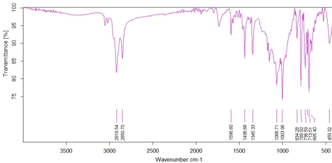
**Figure S4.** IR spectrum (neat, diamond ATR) of **9Ni**
