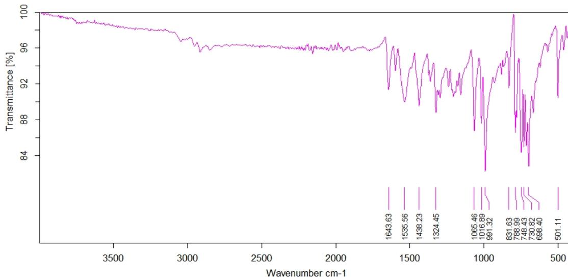
**Figure S16.** IR spectrum (neat, diamond ATR) of **11Ni**
