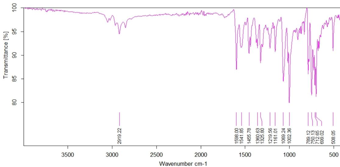
**Figure S26.** IR spectrum (neat, diamond ATR) of **14Ni**
