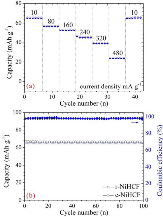
Figure S4. The rate capability of c-NiHCF (a); cycle performance of r-NiHCF and c-NiHCF under current density of 10 mA g<sup>-1</sup> (b).
