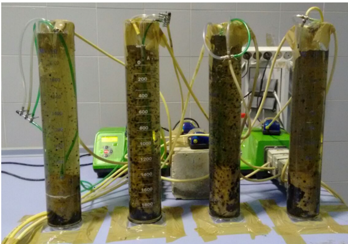
Figure S5. Experimental setup of four laboratory scale CANON bioreactors.
