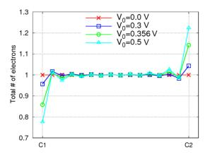
Figure S3. Total number of electrons at each carbon atom along the transverse direction of zGNR.
