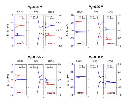
**Figure S1.** Local density of states and band structure of two edge carbon atoms of pristine 8-zGNR for four different transverse electric fields denoted by  $V_0$ .
