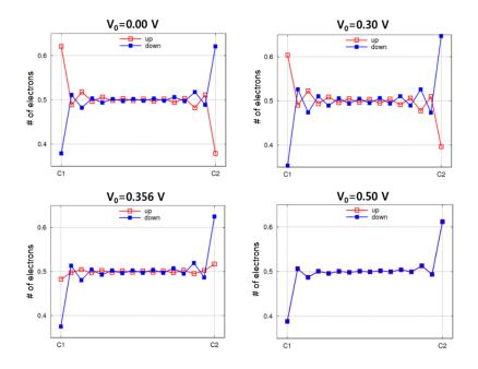
**Figure S2.** The number of spin up and down electrons at each carbon atom along the width of zGNR.
