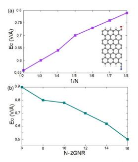
**Figure S4**. Variations of critical electric field (Ec) in terms of (a) coverage fraction of zGNR edges by O-H/C-N groups and (b) width of pristine zGNR. The inset in (a) shows edge modified 8-zGNR with the coverage fraction of 1/4.
