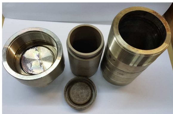
Figure S2. Various components of the autoclave (the metal rod on the right is used for opening and closing the reactor).
