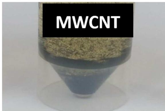
**Figure S6.** Post-digestion MWCNT sample, highlighting the yellowish color of the liquid.
