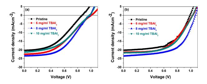
**Figure S1.** (a) Forward and (b) reverse current density-voltage (J-V) characteristics of perovskite solar cells made from pristine and different concentration (6, 8, 10 mg/ml) of TBAI<sub>3</sub> doped perovskite films.
