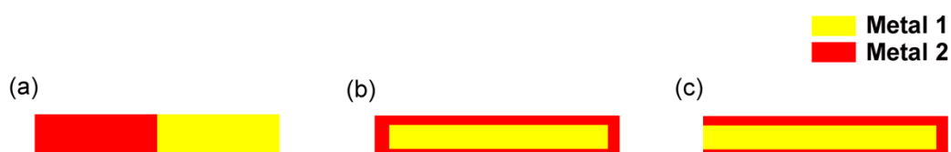
Figure S1. Schematic drawings of three different nanowires: (a) the conventional bimetallic nanowire, (b) the ideal core-shell nanowire, and (c) the core-shell nanowire, studied in this paper.
