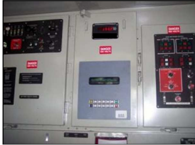
Figure S5. Prime Mover Engine Activity Digital Display in F59PH Locomotive Cab
