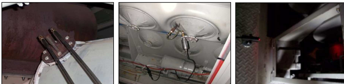
Figure S4. Installation of Sensors on an F59PH Locomotive Prime Mover Engine (a) exhaust sampling port and metal tubes; (b) manifold absolute pressure (MAP) sensor; (c) RPM sensor
