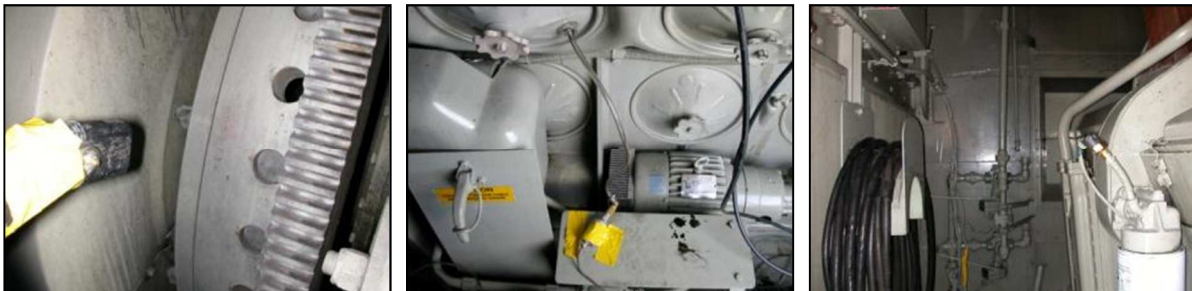
Figure S7. Installation of Sensors on an F59PH Locomotive Prime Mover Engine (a) RPM sensor; (b) manifold absolute pressure (MAP) sensor; (c) intake air temperature (IAT) sensor
