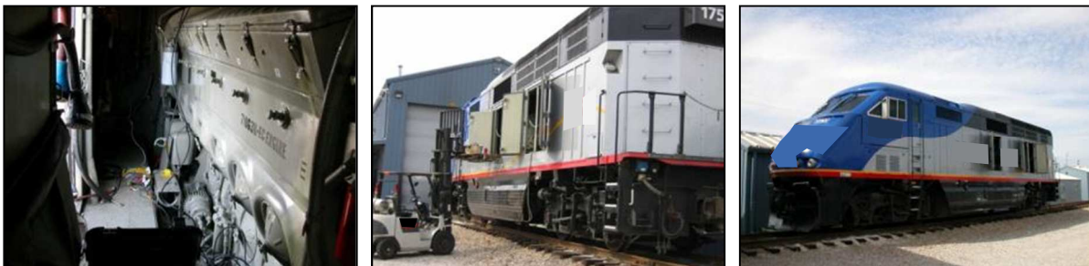
Figure S8. Installation of PEMS Exhaust Sample Lines in an F59PH Locomotive (a) routing sampling hoses and cables; (b) routing sampling hoses through a side door, secured with ties (rear-view); (c) side-view of F59PH locomotive
