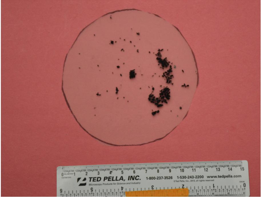
77 **Figure S3.** Image of aged top-load Jacket D 333  $\mu\text{m}$  filter showing the pilling effect of smaller
