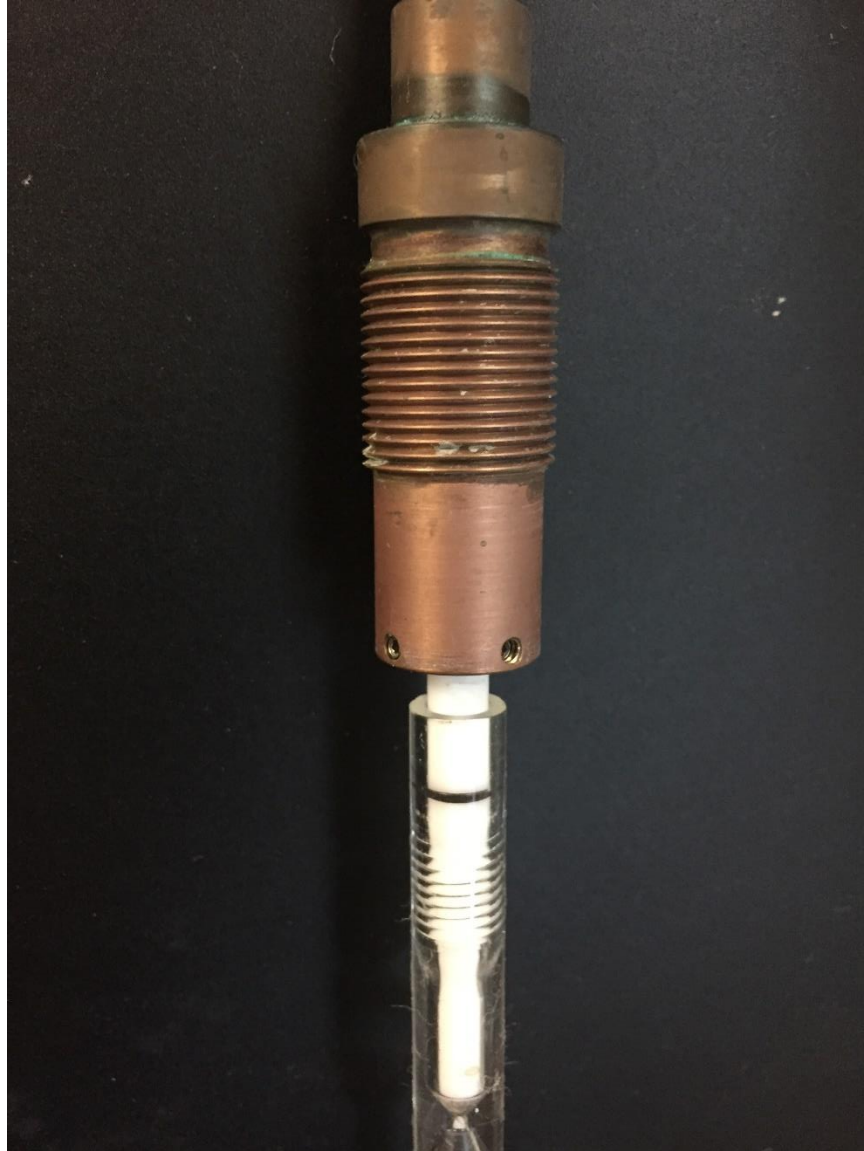
Figure S41. Both set screws tightened. The sample is ready for the plastic protective sleeve.
