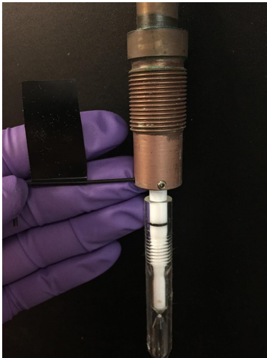
Figure S40. Tightening one of two set screws to secure Teflon pin. By tightening the set screws, the Teflon cap will not be loosened while manipulating sample during pressurization.
