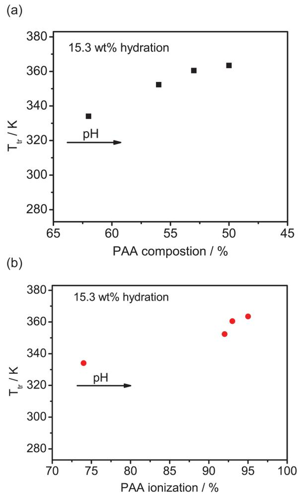
**Figure S6.** (PAH-PAA)<sub>3.5</sub> complex  $T_{tr}$  as a function of (a) PAA composition and (b) PAA ionization.
