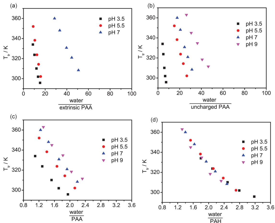
**Figures S5.**  $T_{tr}$  with number of water molecules per (a) extrinsic PAA, (b) neutral PAA, (c) PAA, (d) PAH repeat unit.
