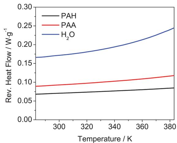
**Figure S4.** MDSC thermograms of 15.3% hydrated homopolymer PAH, PAA and water. The 2<sup>nd</sup> heating scans are shown.
