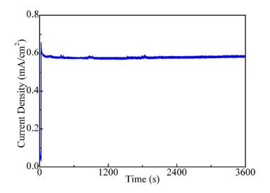
Figure S3. Photocurrent stability for the  $TiO_2/ZnIn_2S_4$  electrode.
