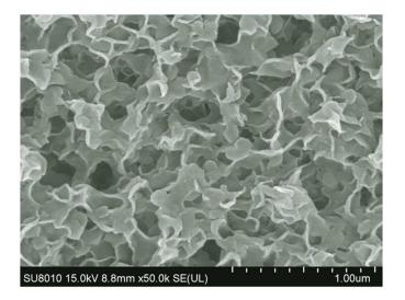
Figure S1. SEM of the top surface view of  $Cu(10s)/TiO_2$ .
