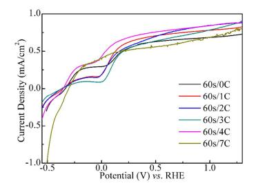
Figure S2. *J-V* curves of Cu(60s)/TiO<sub>2</sub> (0 C) and ZnS-coated Cu(60s)/TiO<sub>2</sub> with different ZnS capping cycles (1 C, 2C, 3C, 4C, 7 C) under one-sun illumination.
