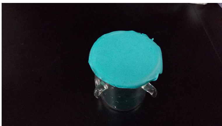
Figure S7. The CEM-8 after 24 h of \text{Cu}^{2+} permeability test.
