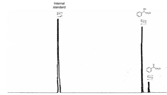
The GC trace for the MPV reduction of  $\alpha$ -chloroacetophenone catalyzed by Me<sub>3</sub>Al
