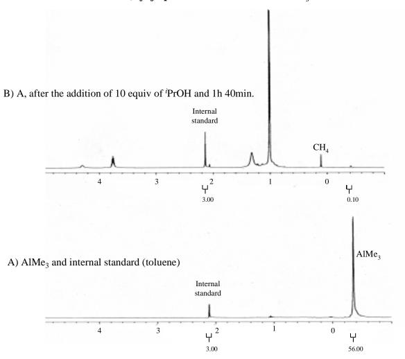
The <sup>1</sup>H NMR(C<sub>6</sub>D<sub>6</sub>) spectra of the reaction of AlMe<sub>3</sub> with <sup>*i*</sup>PrOH
