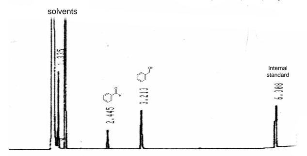
Temp. Program: initial temp. = 90 °C, initial time = 4 min., ramp = 40 °C/min., final temp = 250 °C, final time = 10 min.
