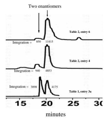
Temp. Program: initial temp. =  $100 \degree C$ , initial time =  $0 \mod r$ , ramp =  $2 \degree C/\min$ , final temp =  $180 \degree C$ , final time =  $10 \min$ .
