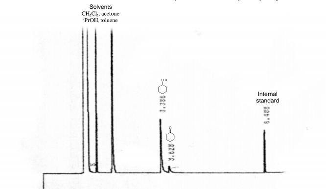
Temp. Program: initial temp. = 60 °C, initial time = 4 min., ramp = 40 °C/min., final temp = 250 °C, final time = 10 min.
