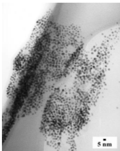
Figure S5. A TEM image of unsupported Au nanoparticles with 1-octadecanethiol ( \text{C}_{18}\text{H}_{37}\text{SH} ).
