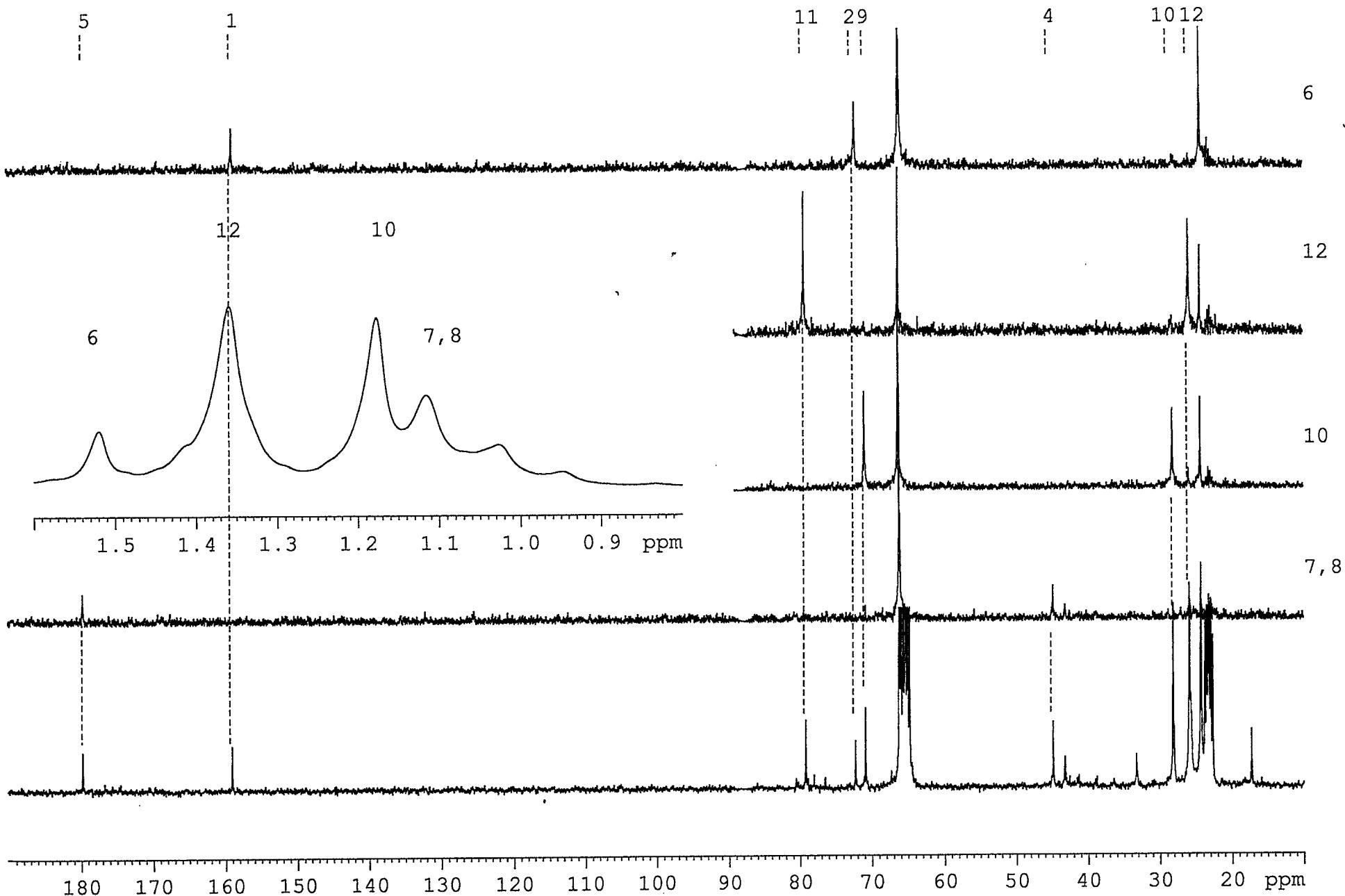
Page 2:  $^{13}\text{C}$  NMR spectrum of the 1:3 A:B mixture with SSLR INEPT spectra
