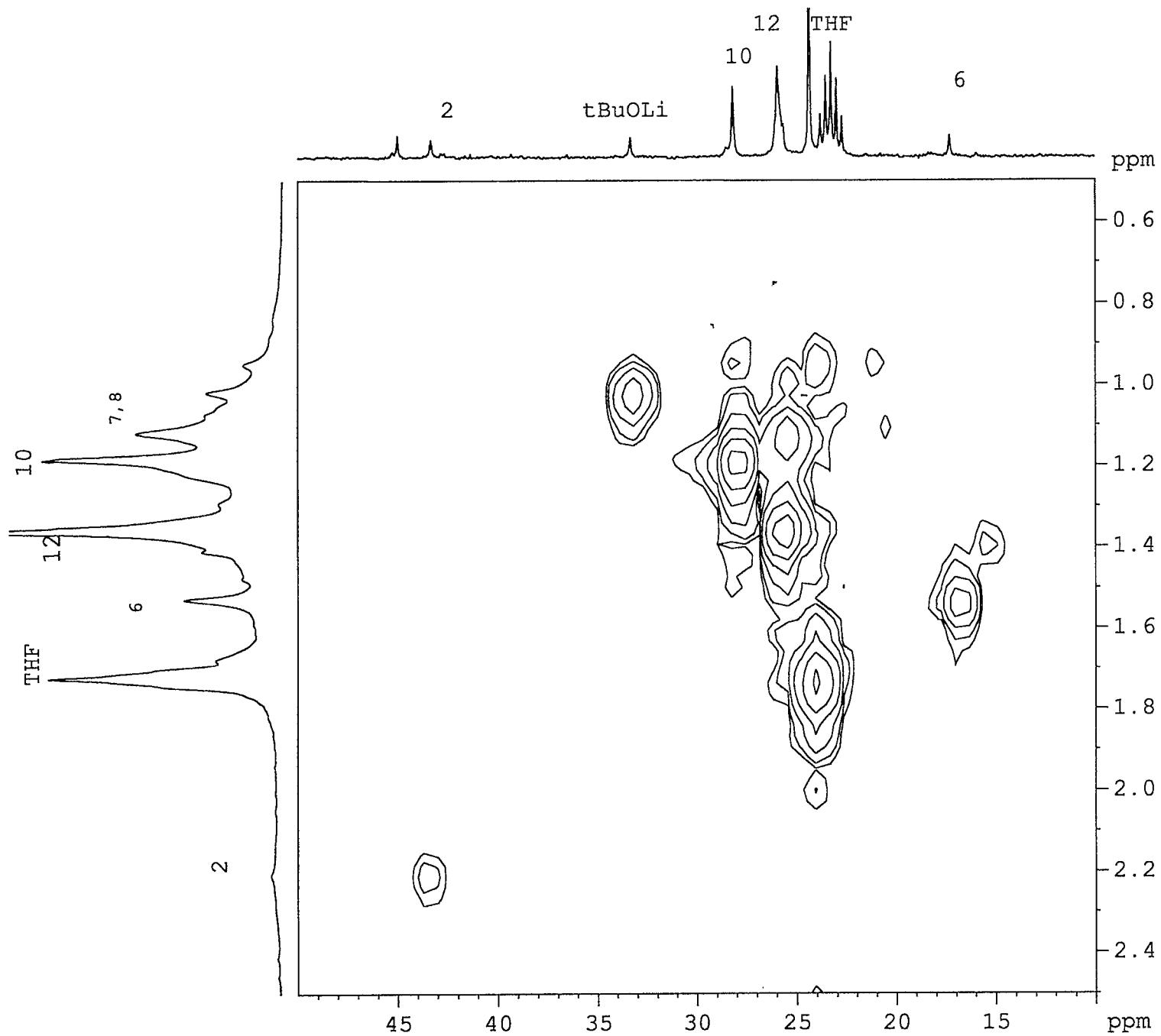
Page 1:  $^1\text{H}$ - $^{13}\text{C}$  COSY(HETCOR) NMR spectrum of the 1:1 A:B mixture at 233K
