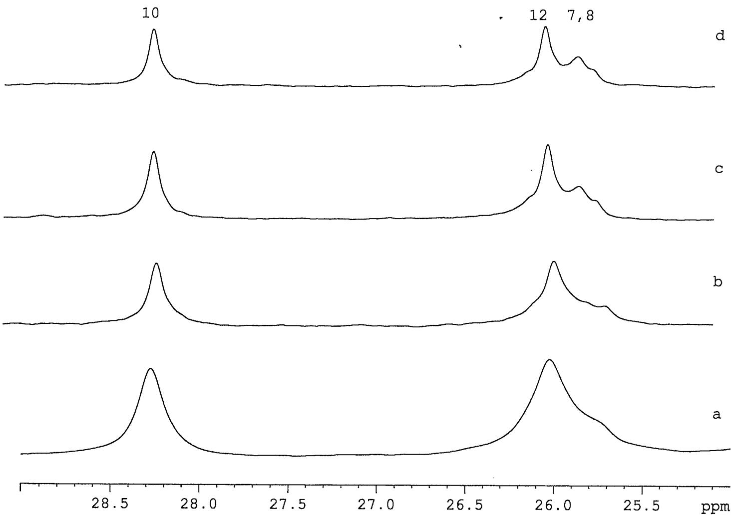
Page 3:  $^{13}\text{C}$  NMR spectra of 1:3 A:B mixture in THF-d<sub>8</sub> (0.3M) at the temperatures 223, 233, 243 and 253 K
