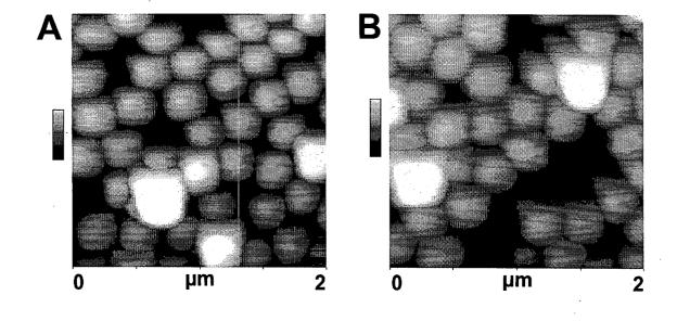
Figure A. Topographic image of latex spheres, showing no changes before and after modifying the tip with 1-dodecylamine. Height bars are  $0.1 \mu m$ . (A) Recorded with an unmodified tip. (B) Recorded with the same tip coated with 1-dodecylamine. After this experiment, the modified tip still exhibited a lower capillary effect than an unmodified tip as determined by our friction measurements.
