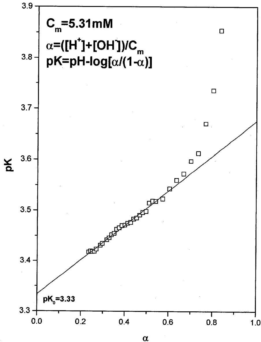
$pK$  values obtained using an extrapolation procedure and the data of a titration experiments.
