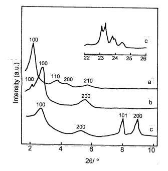
Figure S. XRD patterns of uncalcined samples hydrothermally synthesized at 100°C for 3d (a), 100°C for 3d then 150°C for 3d (b) and 100°C for 3d then 150°C for 3d finally 170°C for 3d (c).
