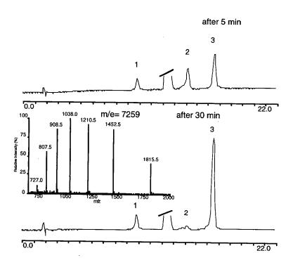
The HPLC chromatogram showing ligation of CI2(1-39)T39D thioester (2) with CI2(40-64)(1) to give the product (3) in 2 hrs.
