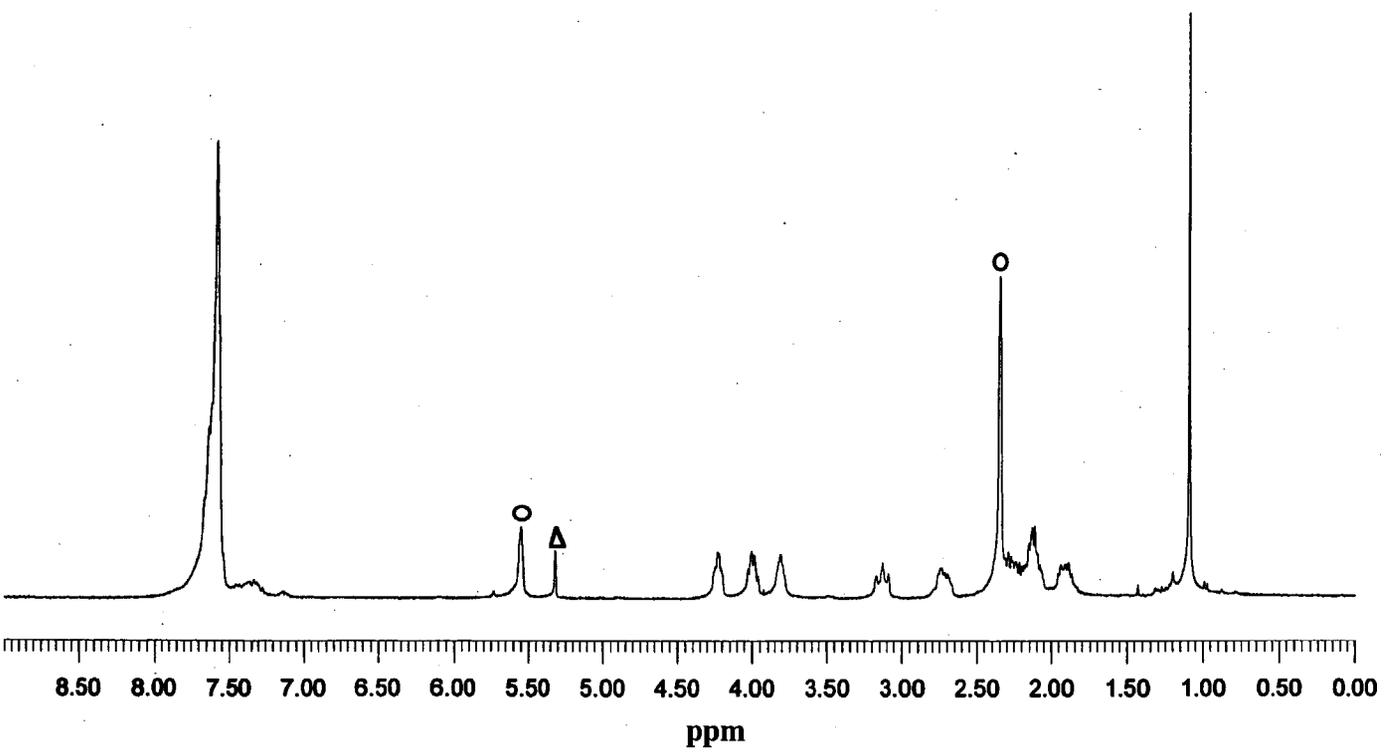
**Figure 3.** 300 MHz <sup>1</sup>H NMR of [Ir((S,S)-DIOP)(COD)]BF<sub>4</sub> in CD<sub>2</sub>Cl<sub>2</sub> at 25°C (O = free COD and Δ = solvent).
