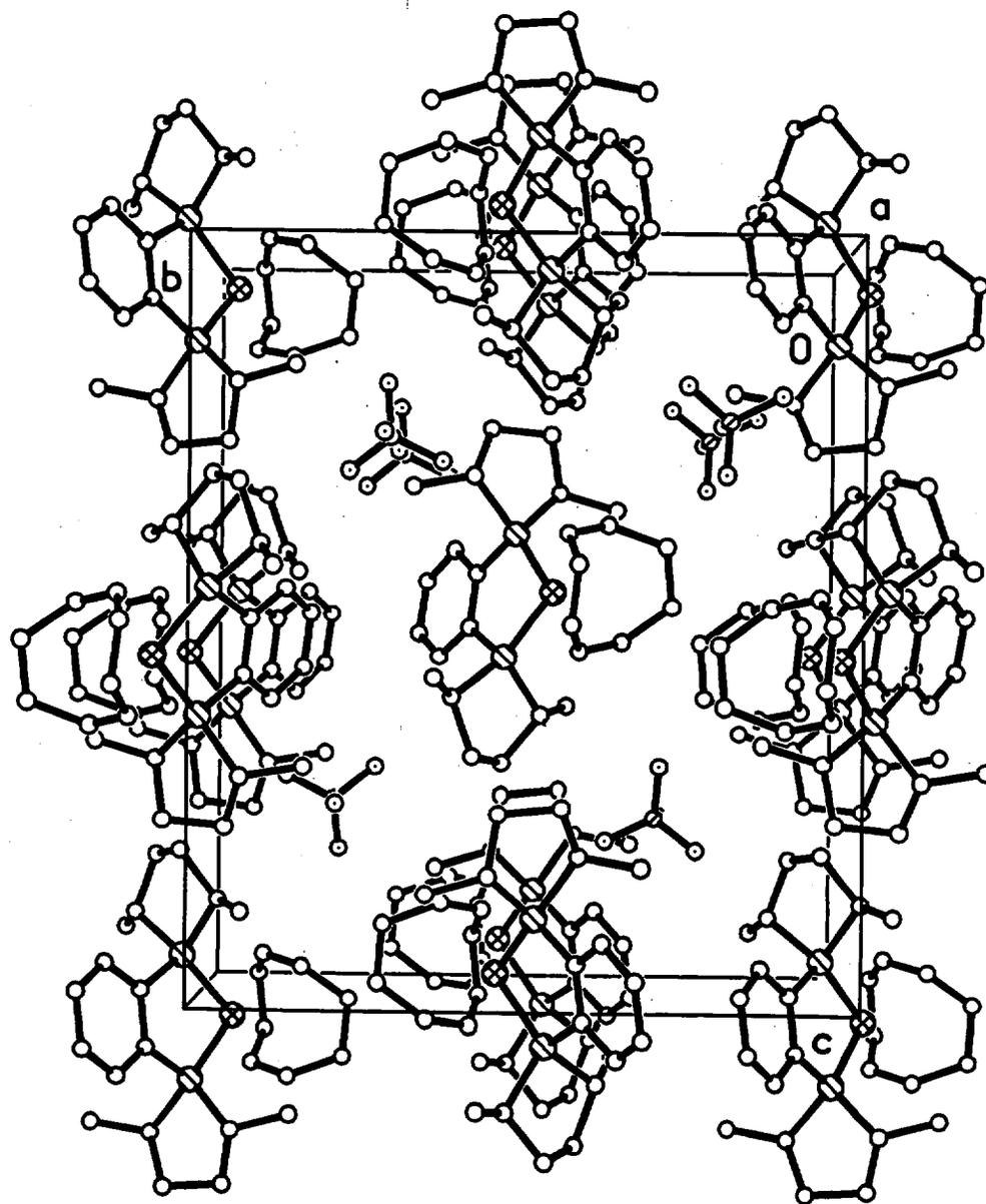
**Figure 2.** Unit cell diagram for  $[\text{Ir}((R,R)\text{-Me-DuPHOS})(\text{COD})]\text{BF}_4$  (5).
