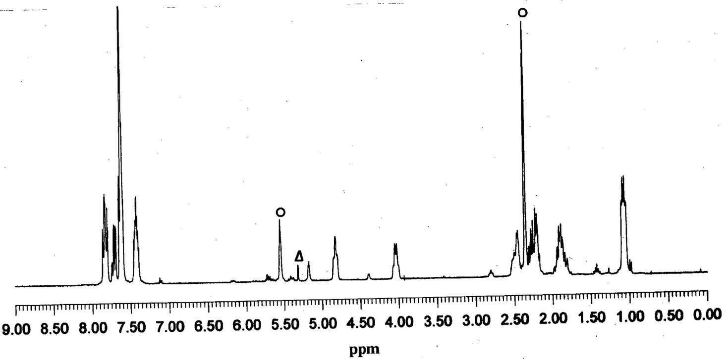
**Figure 4.** 300 MHz  $^1\text{H}$  NMR of  $[\text{Ir}(\text{S},\text{S})\text{-CHIRAPHOS}](\text{COD})(\text{BF}_4)$  in  $\text{CD}_2\text{Cl}_2$  at  $25^\circ\text{C}$
