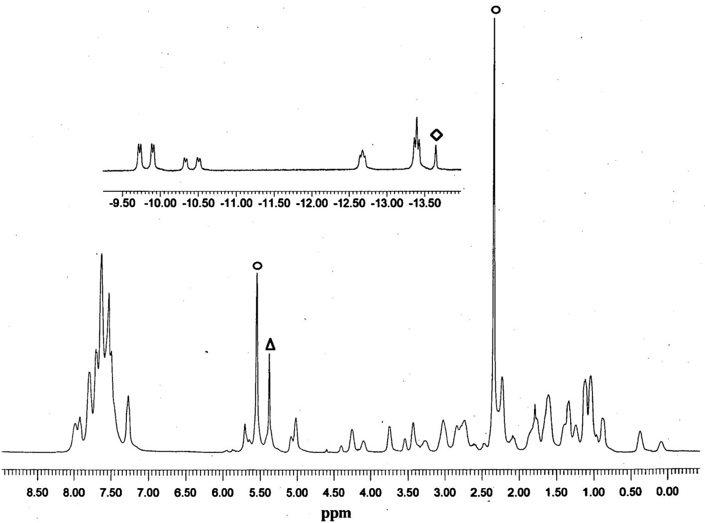
**Figure 11.** 500 MHz <sup>1</sup>H NMR of [IrH<sub>2</sub>((S,S)-CHIRAPHOS)COD]BF<sub>4</sub> in CD<sub>2</sub>Cl<sub>2</sub> at -80°C (O = free COD, ◇ = trace [IrH<sub>2</sub>(COD)<sub>2</sub>]BF<sub>4</sub>, and Δ = solvent).
