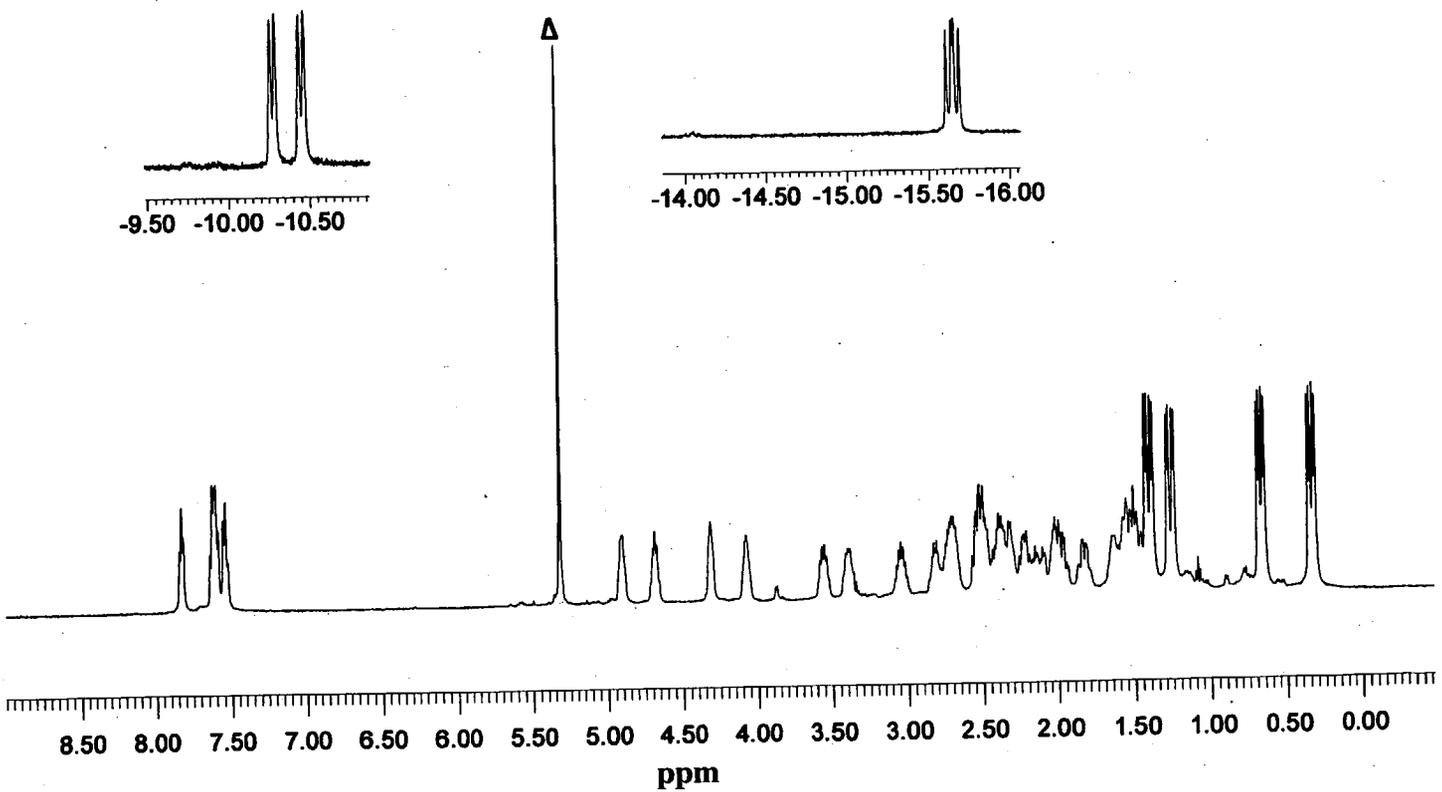
Figure 19. 500 MHz <sup>1</sup>H NMR of [IrH<sub>2</sub>(COD)((R,R)-Me-DuPHOS)]BF<sub>4</sub> in CD<sub>2</sub>Cl<sub>2</sub> at -80°C (Δ = solvent).
