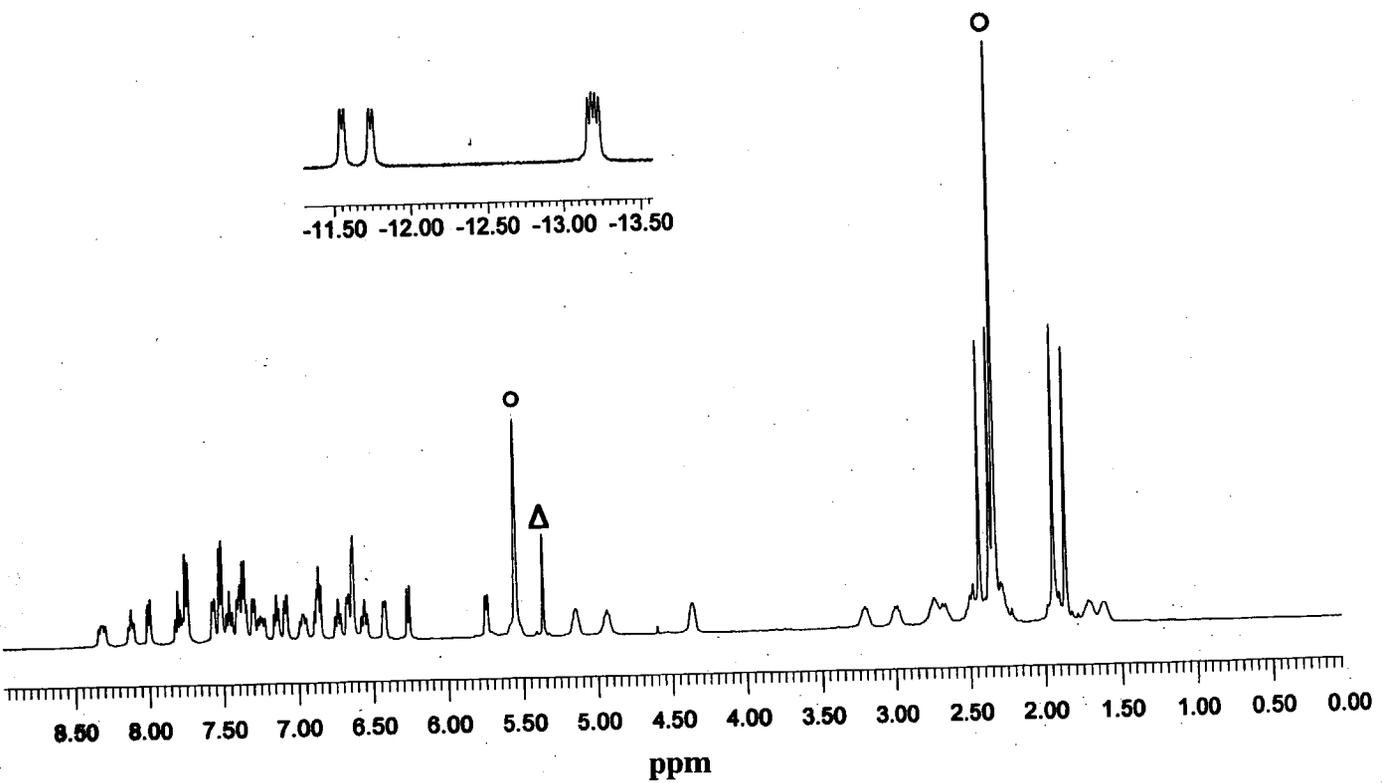
**Figure 13.** 500 MHz <sup>1</sup>H NMR of [IrH<sub>2</sub>((R)-Tol-BINAP)(COD)]BF<sub>4</sub> in CD<sub>2</sub>Cl<sub>2</sub> at -80°C
