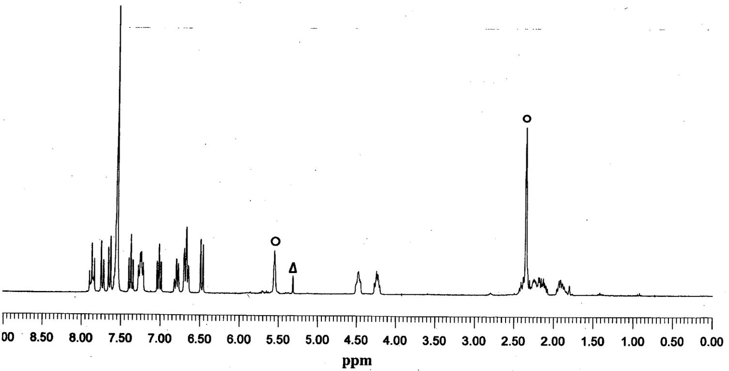
**Figure 5.** 300 MHz  $^1\text{H}$  NMR of  $[\text{Ir}(\text{((R)-BINAP})\text{COD})]\text{BF}_4$  in  $\text{CD}_2\text{Cl}_2$  at  $25^\circ\text{C}$  (O = free COD and  $\Delta$  = solvent).
