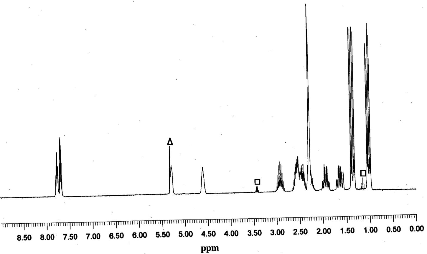
Figure 17. 300 MHz  $^1\text{H}$  NMR of  $[\text{Ir}((R,R)\text{-Me-DuPHOS})(\text{COD})]\text{BF}_4$  in  $\text{CD}_2\text{Cl}_2$  at  $25^\circ\text{C}$  ( $\square$  =  $\text{Et}_2\text{O}$  and  $\Delta$  = solvent).
