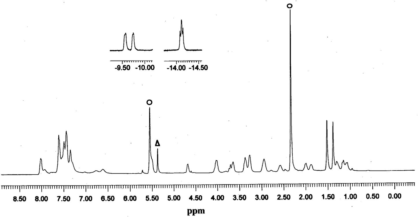
**Figure 10.** 500 MHz <sup>1</sup>H NMR of [IrH<sub>2</sub>((S,S)-DIOP)(COD)]BF<sub>4</sub> in CD<sub>2</sub>Cl<sub>2</sub> at -80°C
