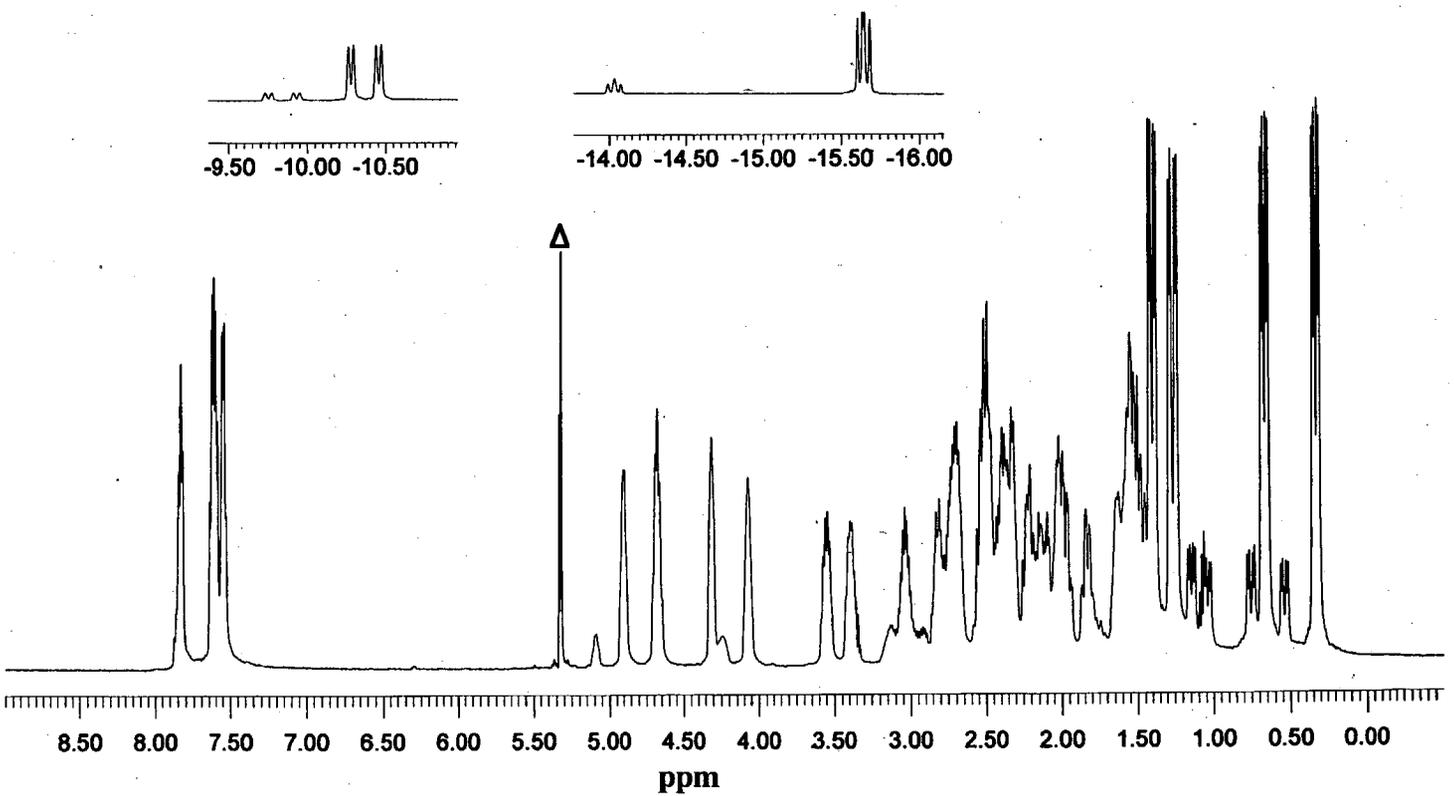
**Figure 21.** 500 MHz <sup>1</sup>H NMR of the equilibrium mixture (reached at -45°C) of  $[\text{TiH}_2(\text{COD})((R,R)\text{-Me-DuPHOS})]\text{BF}_4$  in  $\text{CD}_2\text{Cl}_2$  taken at -80°C (Δ = solvent).
