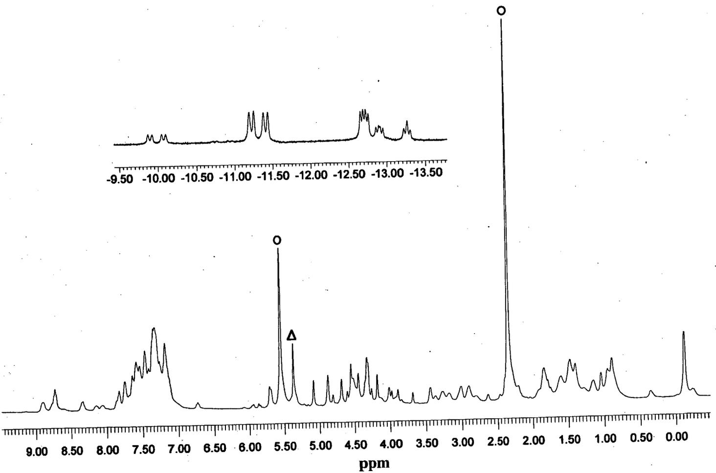
Figure 15. 500 MHz <sup>1</sup>H NMR of [IrH<sub>2</sub>((S,R)-BPPFA)(COD)]BF<sub>4</sub> in CD<sub>2</sub>Cl<sub>2</sub> at -80°C
