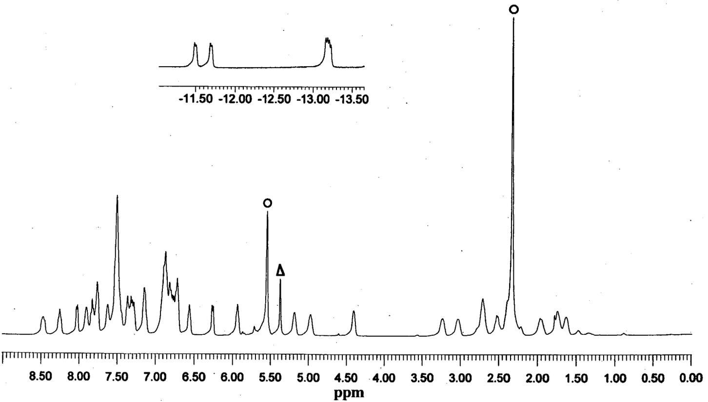
**Figure 12.** 500 MHz <sup>1</sup>H NMR of [TiH<sub>2</sub>((R)-BINAP)(COD)]BF<sub>4</sub> in CD<sub>2</sub>Cl<sub>2</sub> at -80°C (ppm)
