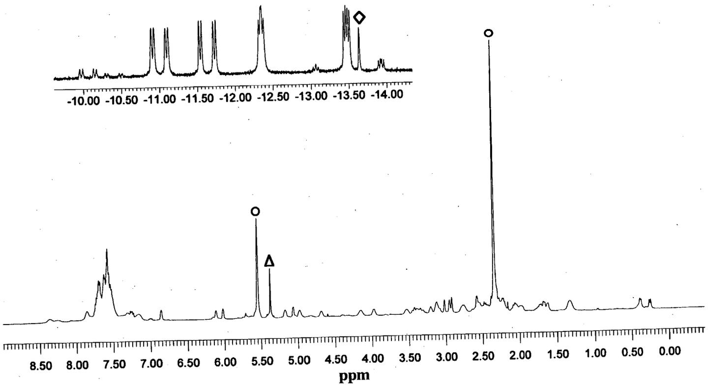
Figure 14. 500 MHz <sup>1</sup>H NMR of [LiH<sub>2</sub>((R,R)-NORPHOS)(COD)]BF<sub>4</sub> in CD<sub>2</sub>Cl<sub>2</sub> at -80°C (O = free COD, ◊ = trace [LiH<sub>2</sub>(COD)]<sub>2</sub>BF<sub>4</sub>, and Δ = solvent).
