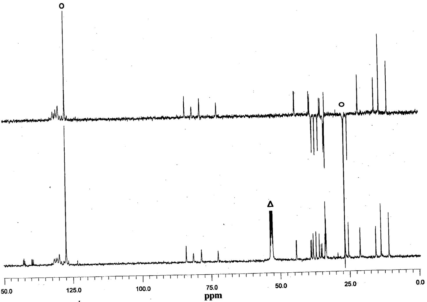
Figure 20. 126 MHz  $^{13}\text{C}$  NMR and DEPT 135 of  $[\text{IrH}_2(\text{COD})]((R,R)\text{-Me-DuPHOS})\text{BF}_4$  in  $\text{CD}_2\text{Cl}_2$  at  $-80^\circ\text{C}$  (O = free COD and  $\Delta$  = solvent).
