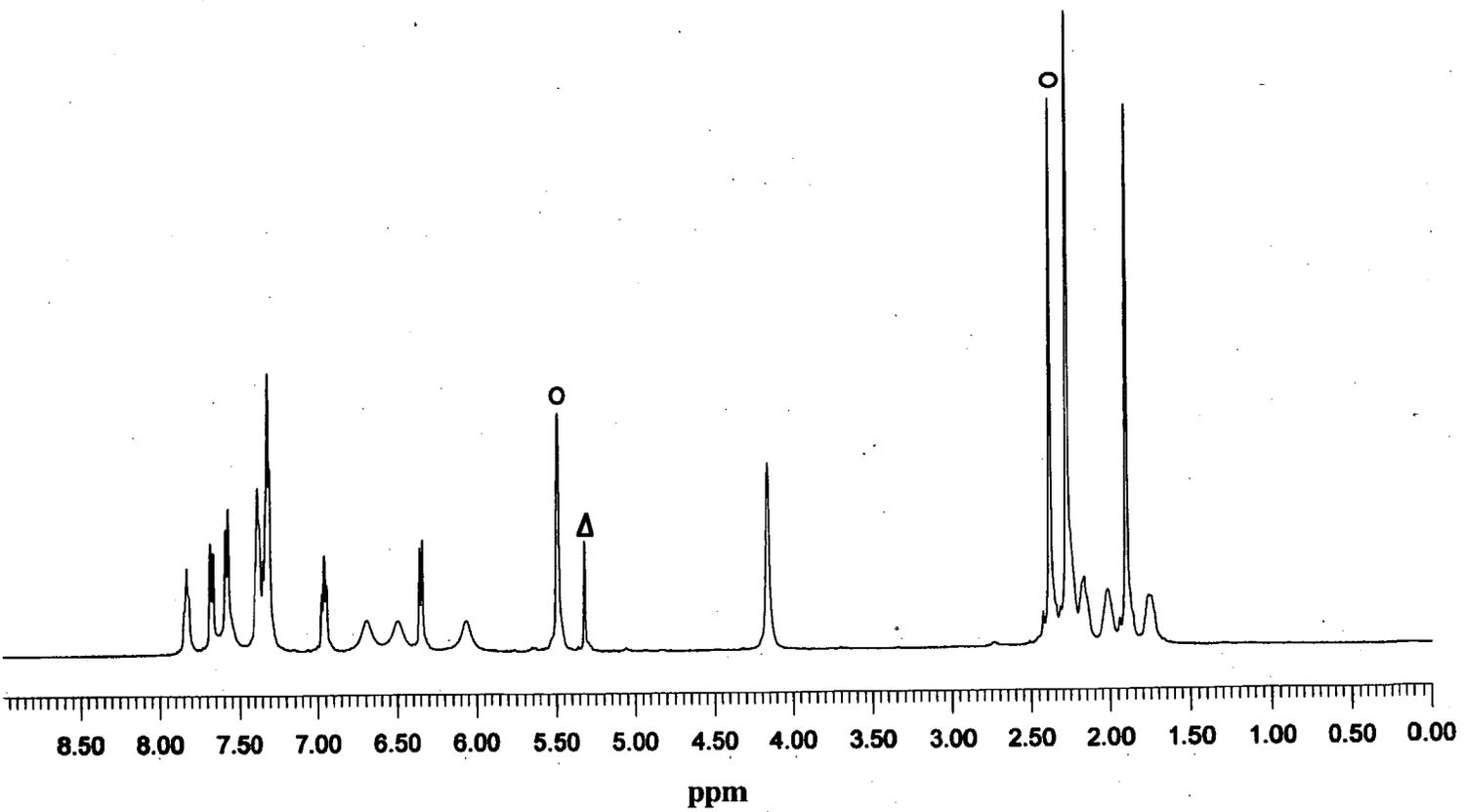
**Figure 6.** 300 MHz <sup>1</sup>H NMR of [Ir((*R*)-Tol-BINAP)(COD)]BF<sub>4</sub> in CD<sub>2</sub>Cl<sub>2</sub> at 25°C (O = free COD and Δ = solvent).
