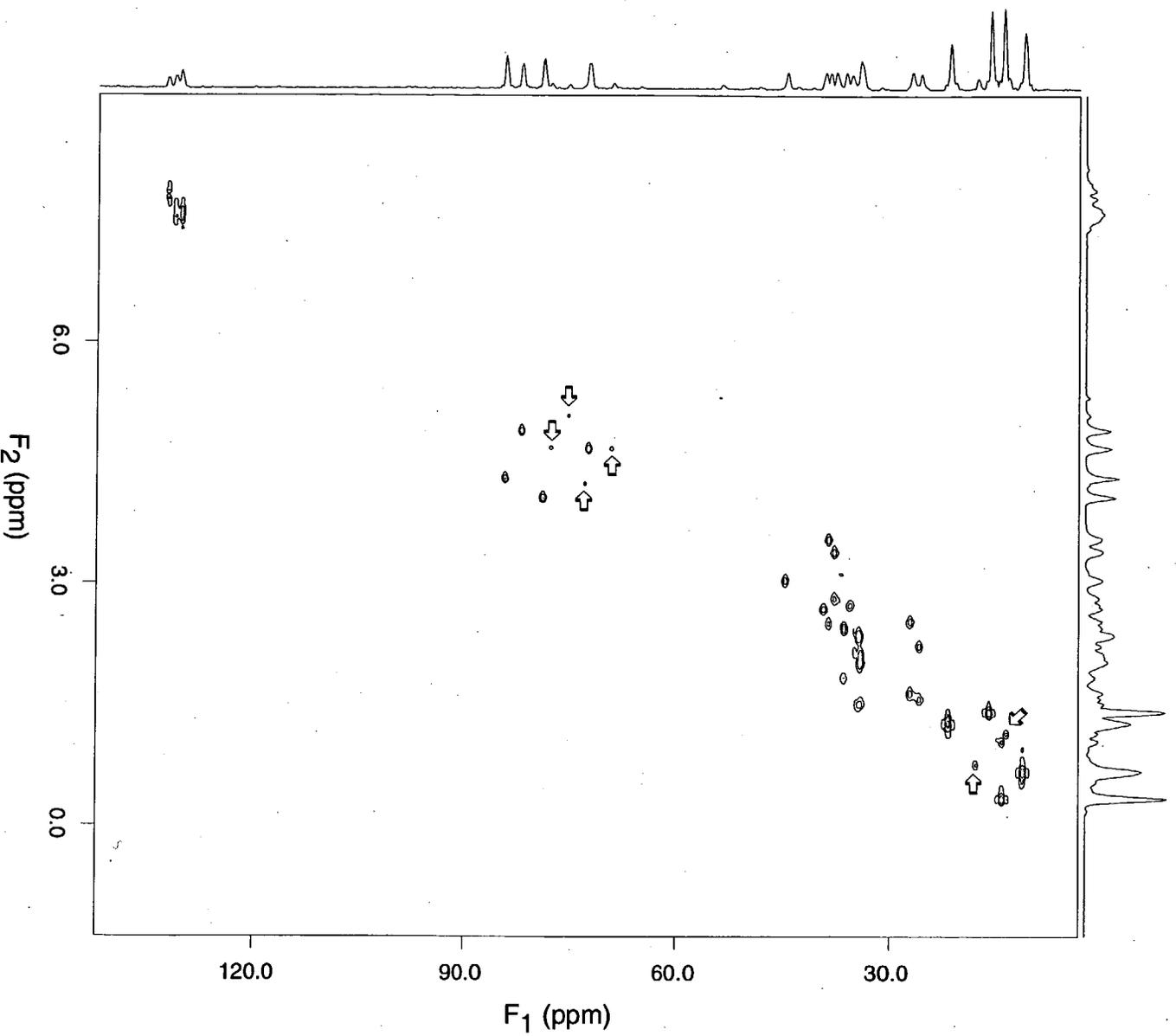
**Figure 25.** 500 MHz  $^1\text{H}$ - $^{13}\text{C}$  HMQC of the equilibrium mixture of  $[\text{IrH}_2(\text{COD})](R,R)\text{-Me-DuPHOS}]\text{BF}_4$ ,  $10^{\text{min}}$ / $10^{\text{min}}$ , at  $-80^\circ\text{C}$  in  $\text{CD}_2\text{Cl}_2$ . The open arrows point to peaks of the minor diastereomer  $10^{\text{min}}$ .
