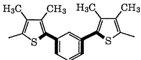
Lowest energy conformers found had both of the thiophene moieties twisted about  $30^\circ$  away from the plane of the phenyl ring.
