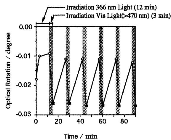
Change of optical rotation of PMMA films doped with
