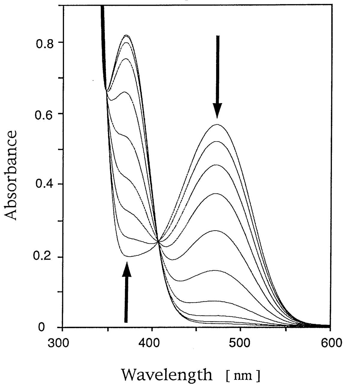
Absorption spectral change of UV-pss of 2( $1.40 \times 10^{-4}$  mol dm $^{-3}$  in toluene. Cell length: 1 cm) to 2E.
