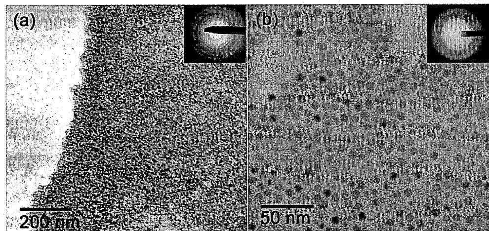
**Figure 3.** Transmission electron micrographs of (a) 10 nm diameter  $\text{TiO}_2$  nanocrystals and (b) 8 nm diameter  $\text{PbTiO}_3$  nanocrystals.
