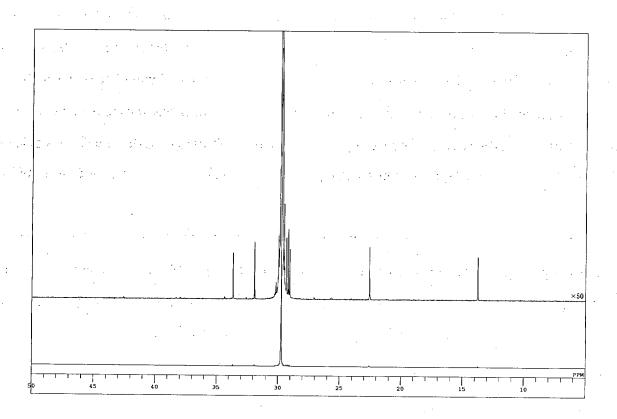
Figure 1. <sup>13</sup>C-NMR spectra of polyethylene produced by complex 1 / MAO
