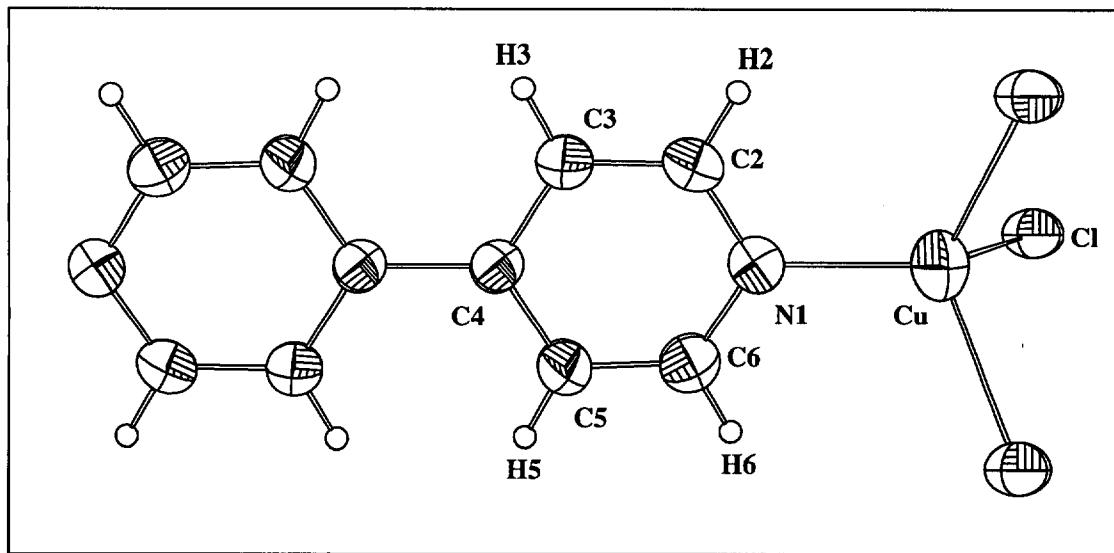
ORTEP drawing of **I** with thermal vibrational ellipsoids (50%)
