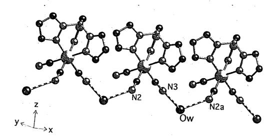
Figure S2. Hydrogen bonds linking the half-sandwich fac-[Fe<sup>III</sup>[HB(pz)<sub>3</sub>](CN)<sub>3</sub>]-anions in complex 1.
