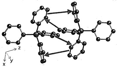
Figure S1. A view of a pair of PPh<sub>4</sub><sup>+</sup> cations in the structure of 1 showing the edge to face interaction between the phenyl rings.
