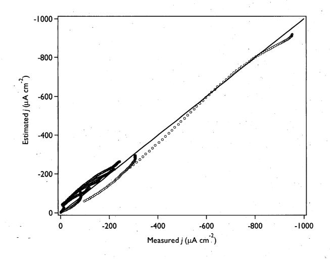
Figure S1. Comparison of estimated and measured current densities. Current densities were calculated with eq 15 and the global parameters given in Table 1. The solid line is given to show a 1:1 slope (i.e., perfect agreement between the model and experimentally measured observations).
