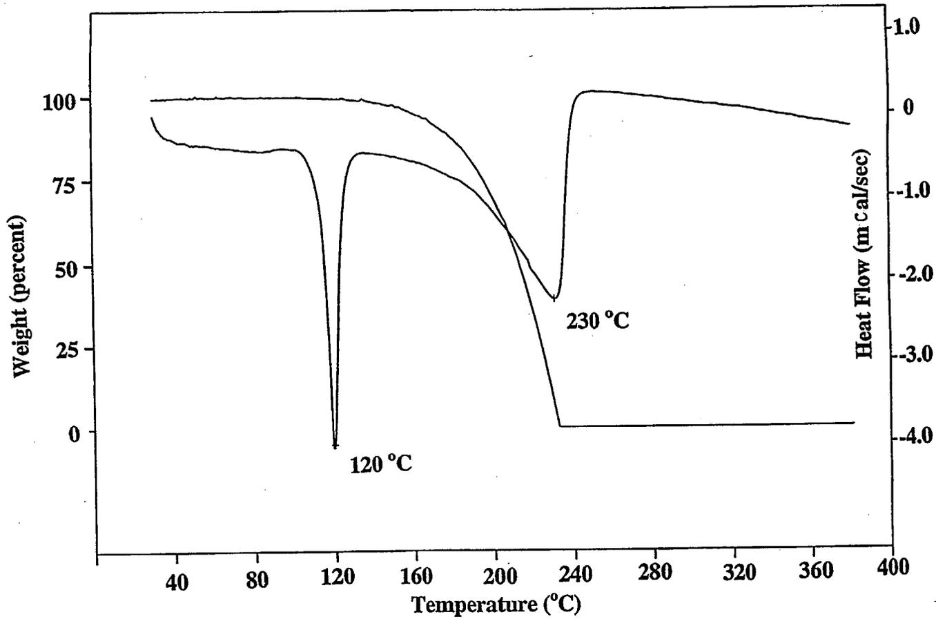
Thermogravimetric analysis (TGA, weight %) and differential scanning calorimetry (DSC, heat flow, mcal/sec) traces for the thermal analysis of (hfac)Ir(1,5-COD).
