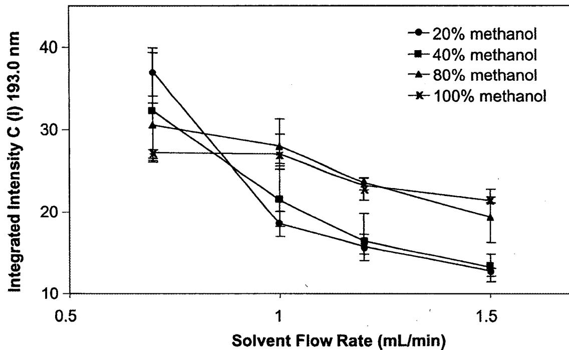
**Figure S1.** Effect of solvent flow rate on C (I) (193.0 nm) emission intensity for triplicate injections of 100  $\mu\text{g}/\text{ml}$  bovine serum albumin in 10% HCl. Solvent flow rate = 1.5 mL/min; nebulizer tip temperature = 280 °C; nebulizer gas flow rate =~800 mL/min; desolvation chamber flow rate =~200 mL/min; HC block temperature = 250 °C; source pressure = 1 Torr He; discharge current = 60 mA.
