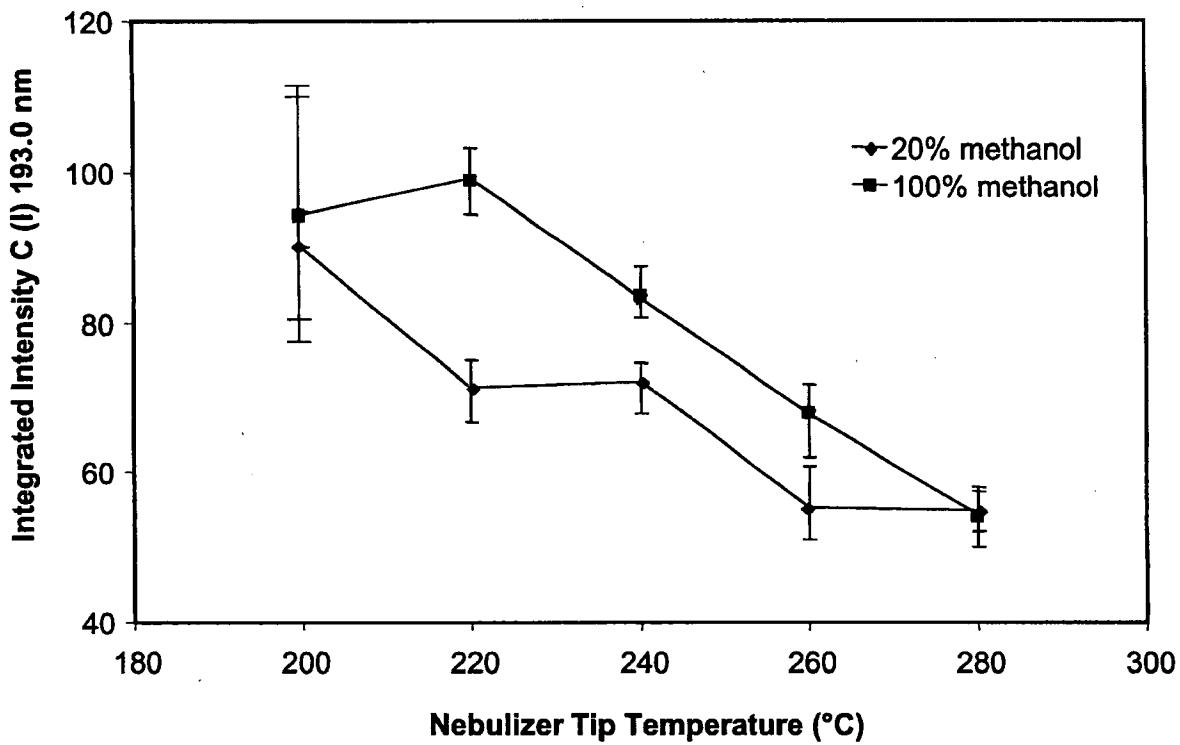
**Figure S2.** Effect of nebulizer tip temperature on C (I) (193.0 nm) emission intensity for triplicate injections of 100  $\mu\text{g}/\text{ml}$  bovine serum albumin in 10% HCl. Solvent flow rate = 0.7 mL/min; nebulizer gas flow rate = ~800 mL/min; desolvation chamber flow rate = ~200 mL/min; HC block temperature = 250 °C; source pressure = 1 Torr He; discharge current = 60 mA.
