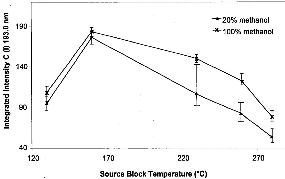
**Figure S4.** Effect of HC source block temperature on C (I) (193.0 nm) emission intensity for triplicate injections of 100 µg/ml bovine serum albumin in 10% HCl. Solvent flow rate = 0.7 mL/min; nebulizer tip temperature = 220 °C; nebulizer gas flow rate =~800 mL/min; desolvation chamber flow rate =~85 mL/min; source pressure = 1 Torr He; discharge current = 60 mA.
