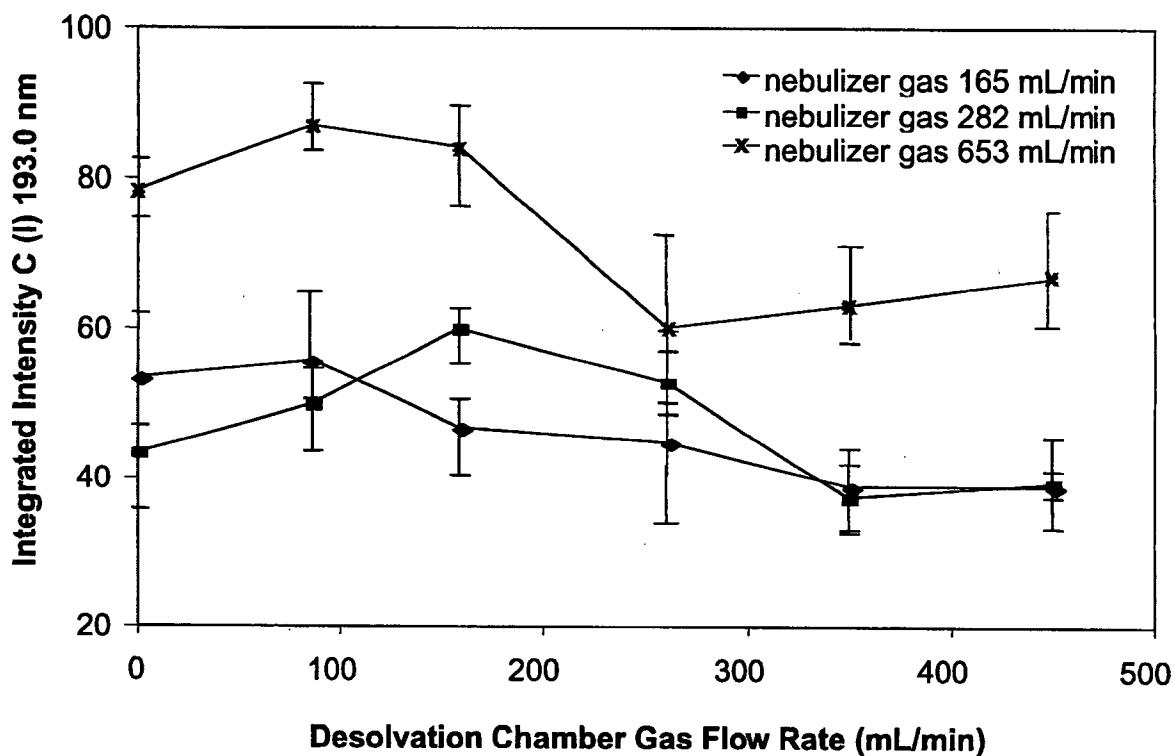
**Figure S3.** Effect of nebulizer gas flow rate and auxiliary spray chamber gas flow rate on C (I) (193.0 nm) emission intensity for triplicate injections of 100  $\mu\text{g}/\text{ml}$  bovine serum albumin in 10% HCl. Solvent flow rate = 0.7 mL/min; nebulizer tip temperature = 220 °C; HC block temperature = 250 °C; source pressure = 1 Torr He; discharge current = 60 mA.
