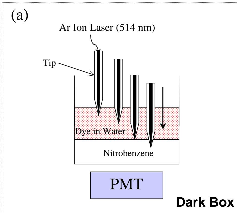
**SI Figure 2.** Schematic of the experimental setup for optical approach.
