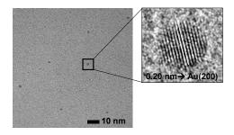
**Figure S1.** Transmission electron microscope (TEM) images of Au nanoparticles (NPs) on a carbon film, grown in the identical conditions for the preparation of the Au NPs on our MoS<sub>2</sub> thin films. The lattice spacing found from the high-resolution TEM image is identified to be around 0.20 nm, corresponding to the Au (200) atomic plane.
