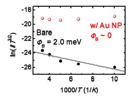
Figure S2. The current (I)-voltage (V) characteristics of our device can be explained by the 2D thermionic model, as described by the following equation:
