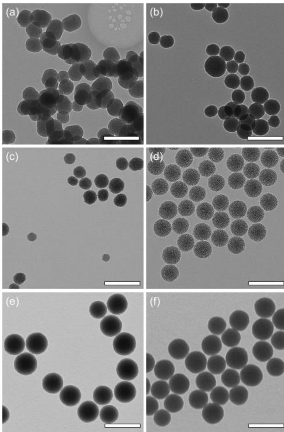
**Figure S1.** TEM images of the silica nanoparticles. a) MCM-41, b) MCM-48S, c) MCM-48R, d) Dendritic, e) Random, and f) SiNP. Scale bars are 250 nm.
