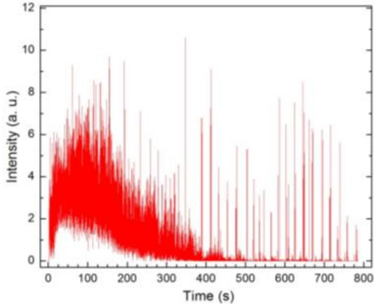
**Figure S4.** Response of MCM-48R ( $10^{11}$  particles  $\text{mL}^{-1}$ ) under continuous HIFU exposure (10.6 MPa) for approximately 13 min.
