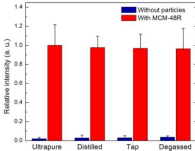
**Figure S5.** The relative intensity generated by the MCM-48R in different types of water. Particle concentration was  $10^{11}$  particles  $\text{mL}^{-1}$  and peak negative pressure was 10.6 MPa. Error bars = 1 SD, studies were run in triplicate.
