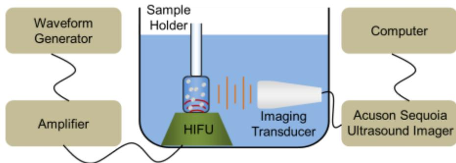
**Figure S2.** Schematic representation of the experimental set-up used for the acoustic cavitation experiments.
