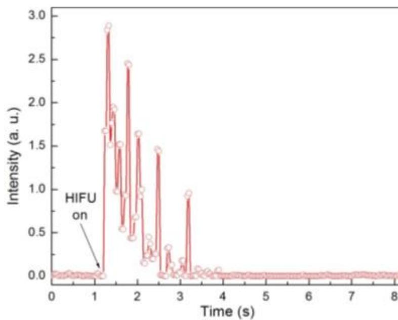
**Figure S3.** Response of Random ( $4 \times 10^{11}$  particles  $\text{mL}^{-1}$ ) under continuous HIFU exposure (10.6 MPa) for approximately 7 s.
