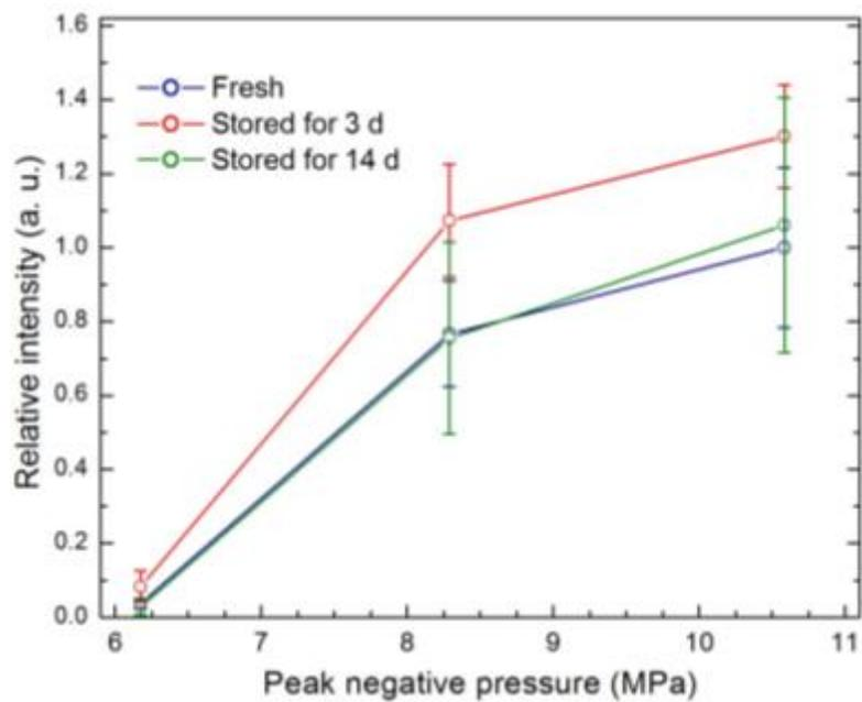
**Figure S6.** Relative response of as dispersed (fresh) and stored (in water, for 3 or 14 d) MCM-48R samples ( $4 \times 10^{11}$  particles  $\text{mL}^{-1}$ ) at different pressures. Error bars = 1 SD, studies were run in triplicate.
