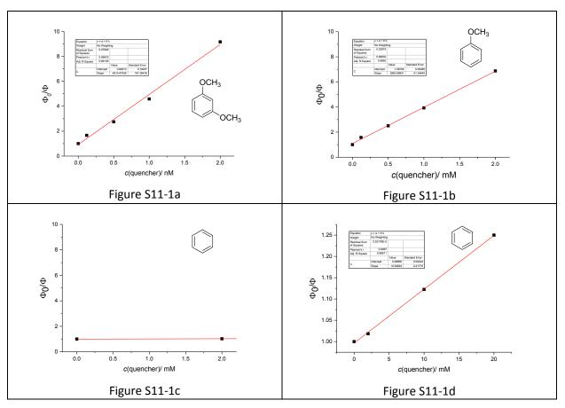
Effective quenching of **3b**-photocycloreversion mediated by catalyst **2c** was observed using quenchers (anisole and 1,3-dimethoxybenzene) with lower oxidation potentials<sup>11</sup> compared to **3b** ( $E^{ox} = 2.05$  V vs SCE). On the other hand benzene<sup>12</sup> having higher oxidation potential did not almost cause quenching of photocycloreversion (see Figure S11-2).
