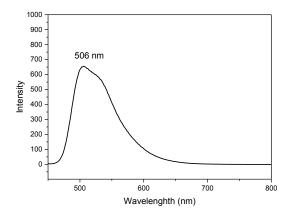
UV-VIS spectrum of **1**+**TfOH** in acetonitrile ( $c(1) = 1 \times 10^{-5}$  M; c(TfOH) = 0.01 M)
