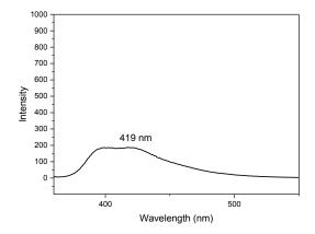
UV-VIS spectrum of **2a** in acetonitrile ( $c(2\mathbf{a}) = 3.75 \times 10^{-5} \text{ M}$ )
