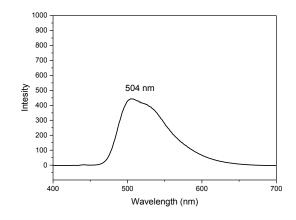
UV-VIS spectrum of **5**+**TfOH** in acetonitrile ( $c(5) = 1 \times 10^{-5}$  M; c(TfOH) = 0.01 M)
