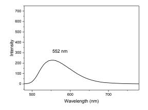
UV-VIS spectrum of **2b** in acetonitrile ( $c(2b) = 3.75 \times 10^{-5}$  M)
