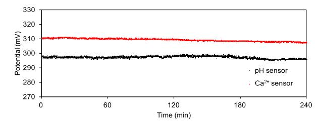
Figure S1. Long-term stability of  $Ca^{2+}$  and pH sensors in 0.01 M acetate buffer containing 1 mM  $CaCl_2$  in 4 hours. Potential is reported with respect to a standard Ag/AgCl reference electrode.
